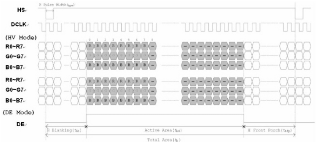
Horizontal input timing diagram
