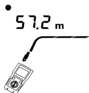
Figure 6.15 Open on Coaxial Cabling
