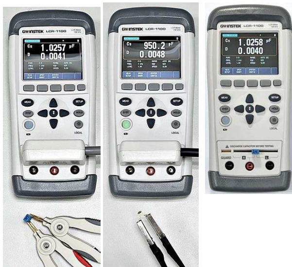
Figure Test results for capacitors
