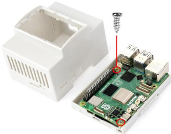
3. fix the Raspberry Pi onto the bottom panel by screws
