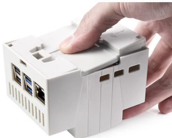
4. put on the bottom panel, aligning it with the buckle and USB connectors
