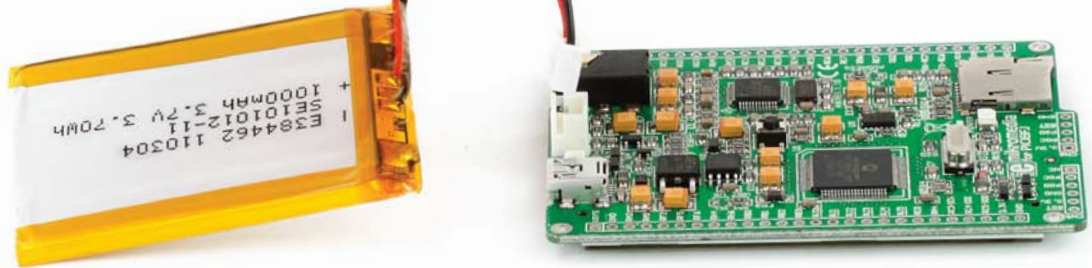
Figure 2-1: Connecting Li-polymer battery to mikromedia™ board
