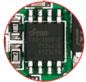
Figure 11-2: Flash memory module
