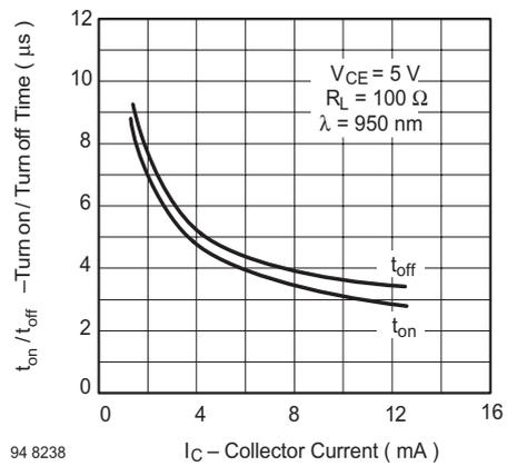
Figure 7. Turn On/Turn Off Time vs. Collector Current
