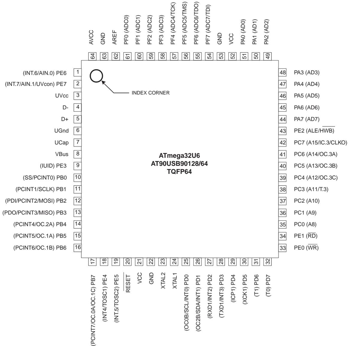
**Figure 1-2.** Pinout ATmega32U6/AT90USB64/128-QFN
