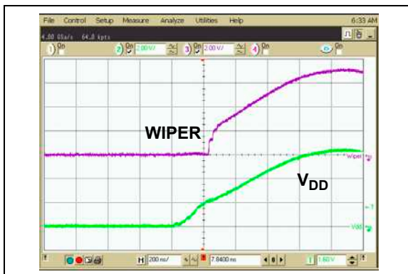
FIGURE 2-52: 50 k\Omega – Power-Up Wiper Response Time.
