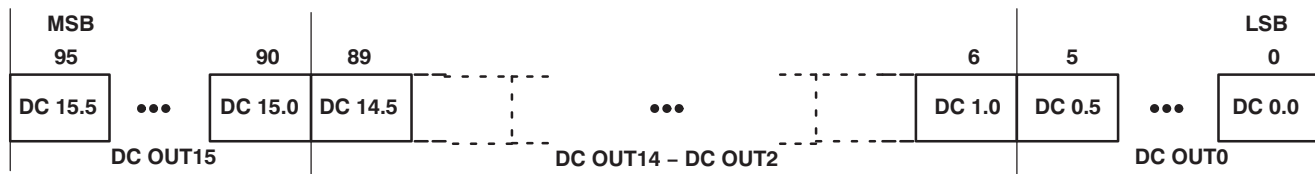
Figure 14. Dot Correction Data Packet Format
