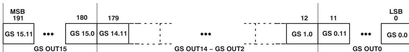
Figure 18. Grayscale Data Packet Format
