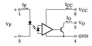
(Note) A  $0.1\mu F$  bypass capacitor must be connected between pins 4 and 6.
