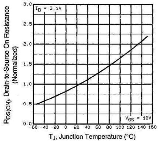
**Fig 4.** Normalized On-Resistance
