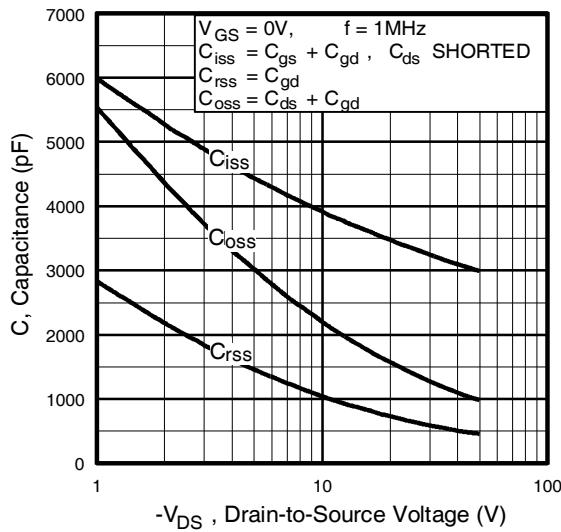
**Fig 5.** Typical Capacitance Vs.
