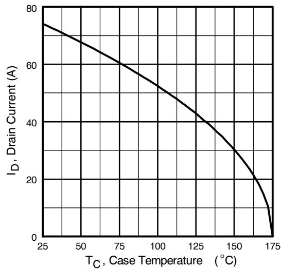
**Fig 9.** Maximum Drain Current Vs.
