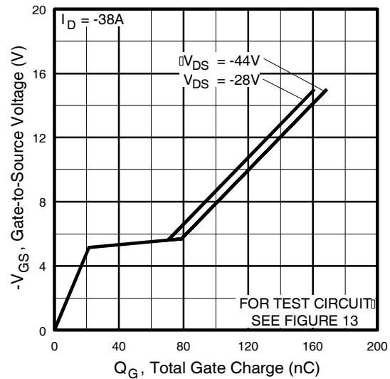
**Fig 6.** Typical Gate Charge Vs.
