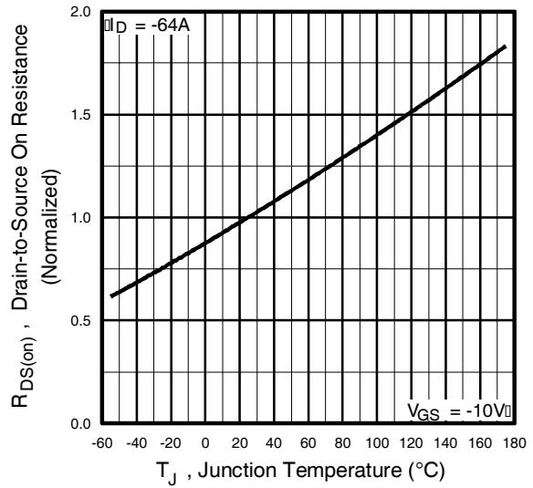
**Fig 4.** Normalized On-Resistance
