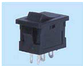
RSSM1013 + LED ON-OFF 10 A 125 VAC; 3 A 250 VAC SPST 4P
