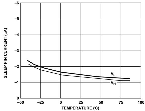
Figure 8.  $\overline{\text{SLEEP}}$  Pin Current vs. Temperature
