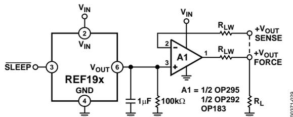
Figure 29. A Low Dropout, Kelvin-Connected Voltage Reference
