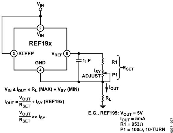
Figure 27. A Low Dropout, Precision Current Source
