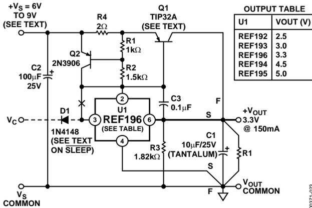
Figure 23 Boosted 3.3 V Referenced with Current Limiting
