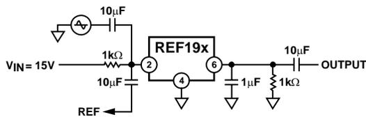
Figure 10. Ripple Rejection vs. Frequency Measurement Circuit
