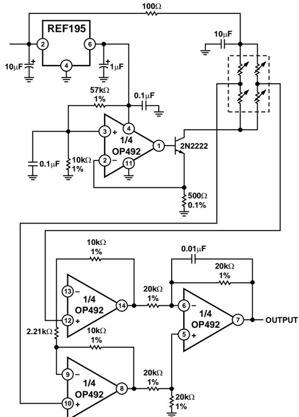
Figure 31. A Low Power, Strain Gage Circuit
