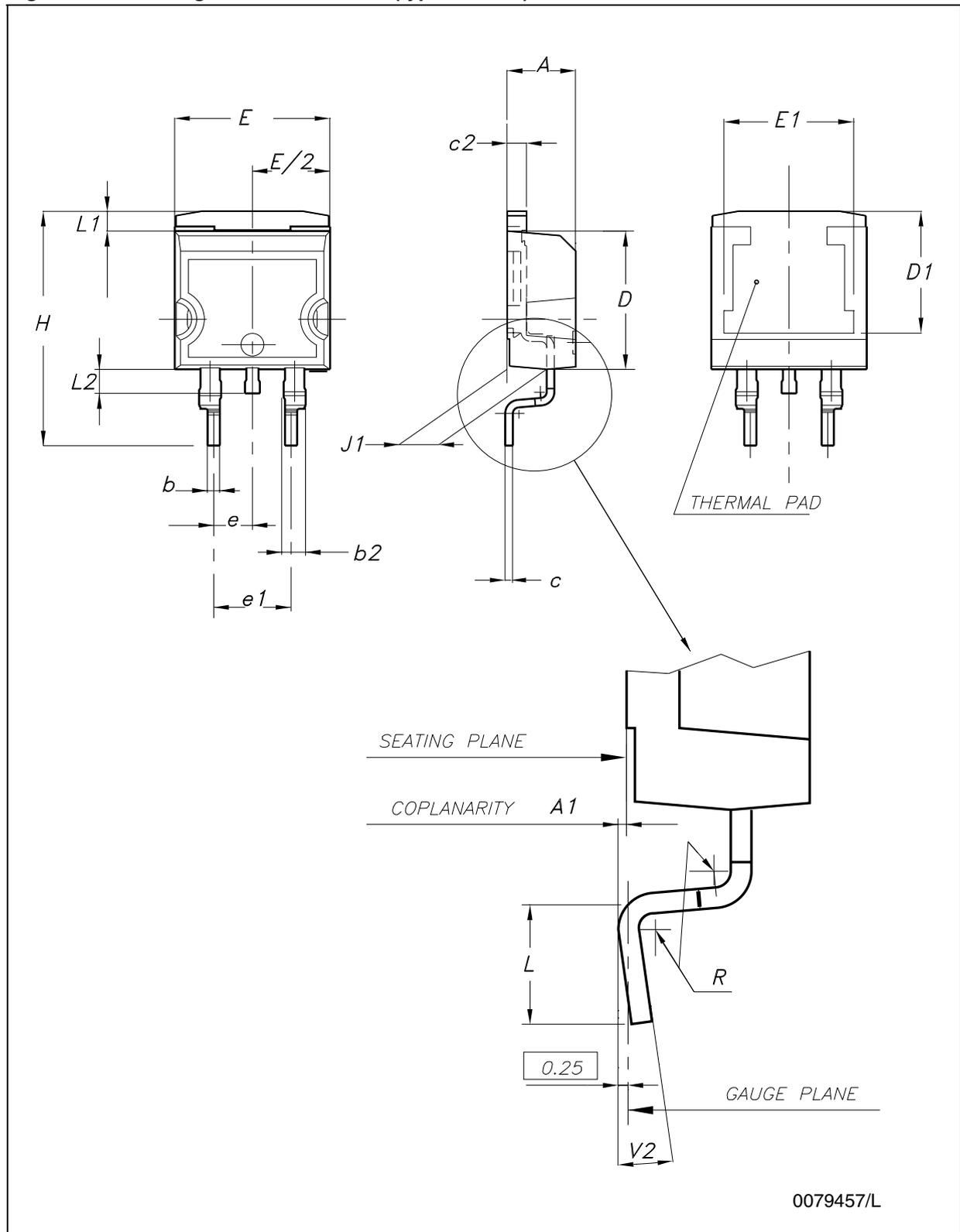
Figure 17. Drawing dimension D<sup>2</sup>PAK (type WOOSEOK-SUBCON.)
