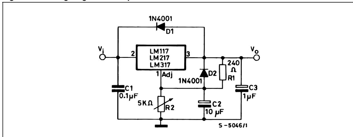
*Note:* D1 protect the device against input short circuit, while D2 protects against output short circuit for capacitors discharging.
