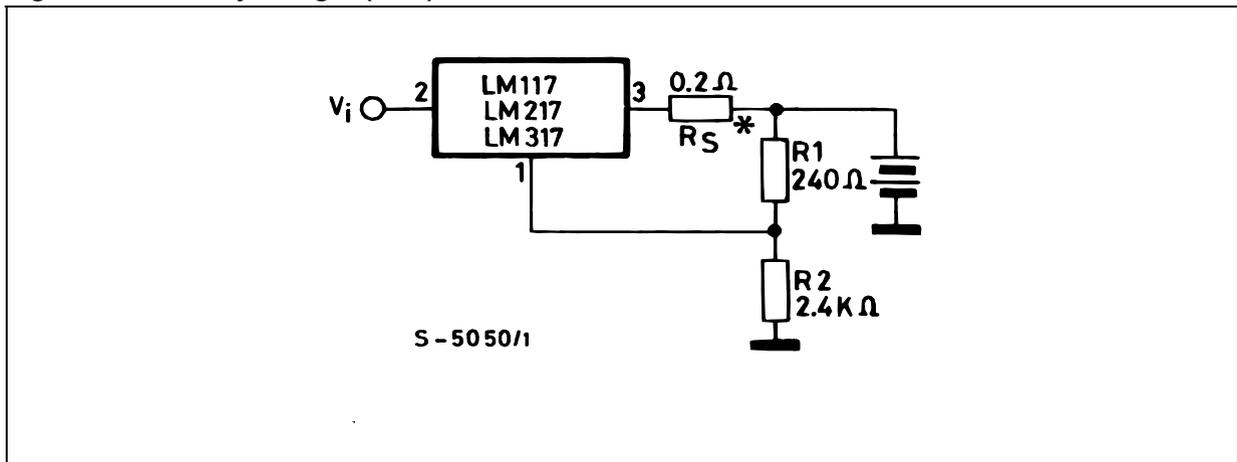
\* R<sub>S</sub> sets output impedance of charger  $Z_O = R_S (1 + R_2/R_1)$ . Use of R<sub>S</sub> allows low charging rates whit fully charged battery.
