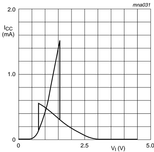
Fig 12. Typical 74HCT1G14 transfer characteristics; V<sub>CC</sub> = 4.5 V
