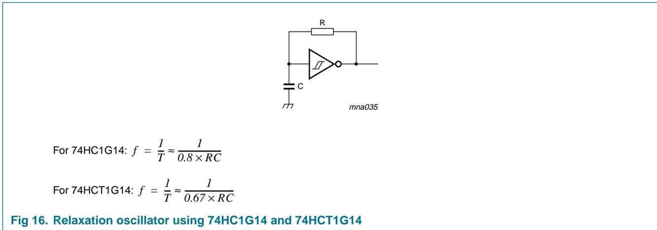
Fig 16. Relaxation oscillator using 74HC1G14 and 74HCT1G14
