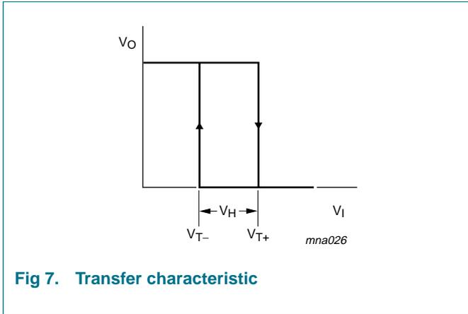
Fig 7. Transfer characteristic
