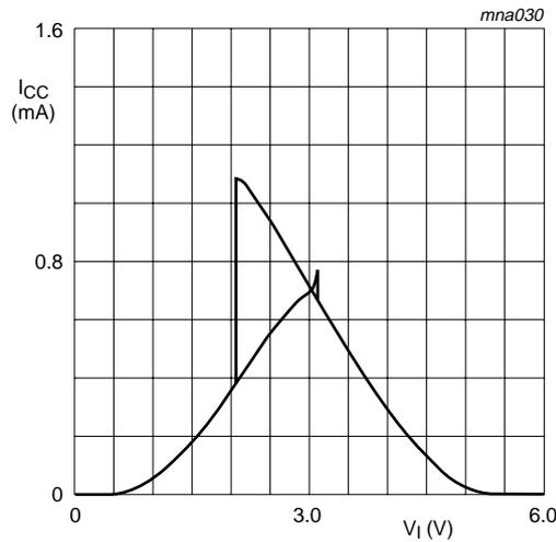
Fig 11. Typical 74HC1G14 transfer characteristics; V<sub>CC</sub> = 6.0 V
