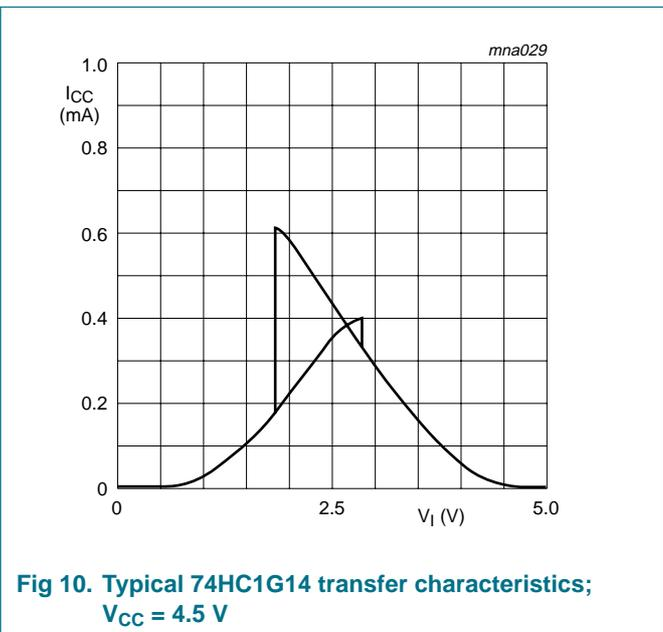
Fig 10. Typical 74HC1G14 transfer characteristics;  $V_{CC} = 4.5$  V
