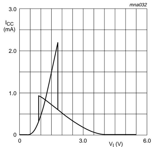
Fig 13. Typical 74HCT1G14 transfer characteristics; V<sub>CC</sub> = 5.5 V
