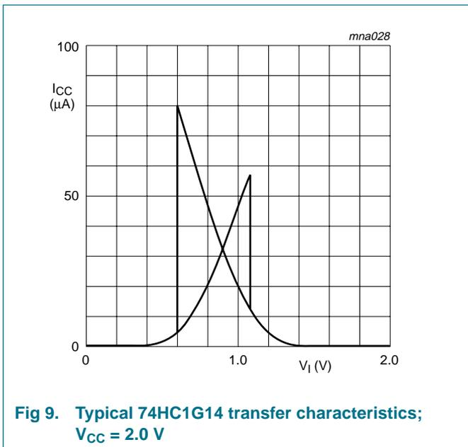
Fig 9. Typical 74HC1G14 transfer characteristics;  $V_{CC} = 2.0$  V
