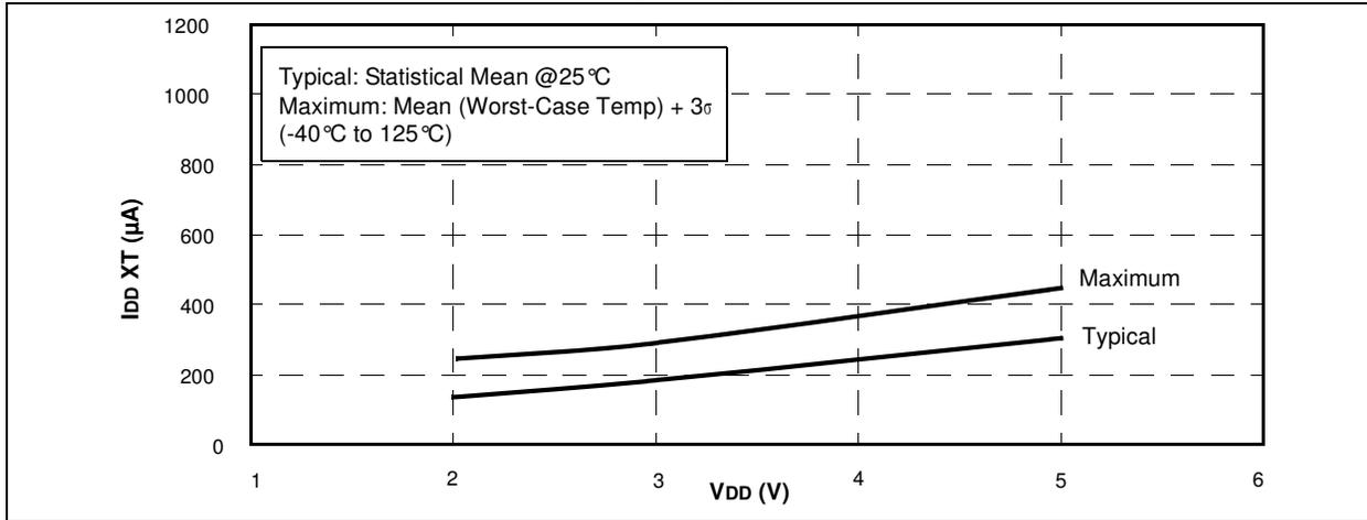
**FIGURE 17-5: PIC12F609/615/617 I<sub>DD XT</sub> (4 MHz) vs. V<sub>DD</sub>**
