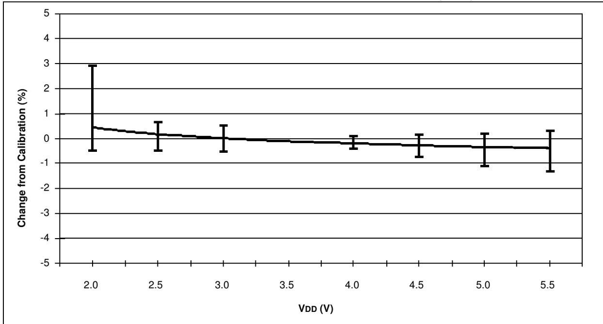
FIGURE 17-44: TYPICAL HFINTOSC FREQUENCY CHANGE vs.  $V_{DD}$  (85 °C)
