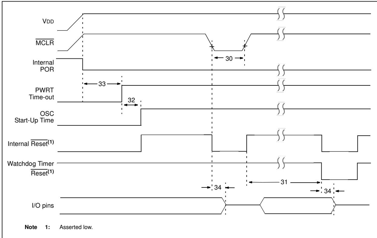
**FIGURE 16-7: BROWN-OUT RESET TIMING AND CHARACTERISTICS**
