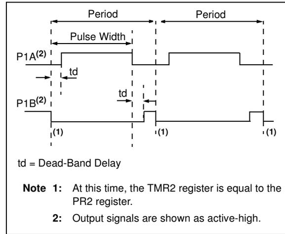
**FIGURE 11-14: EXAMPLE OF HALF-BRIDGE APPLICATIONS**
