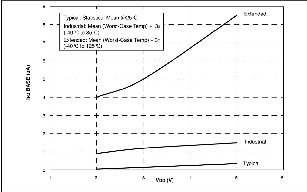
FIGURE 17-11: PIC12F609/615/617 IPD COMPARATOR (SINGLE ON) vs. VDD
