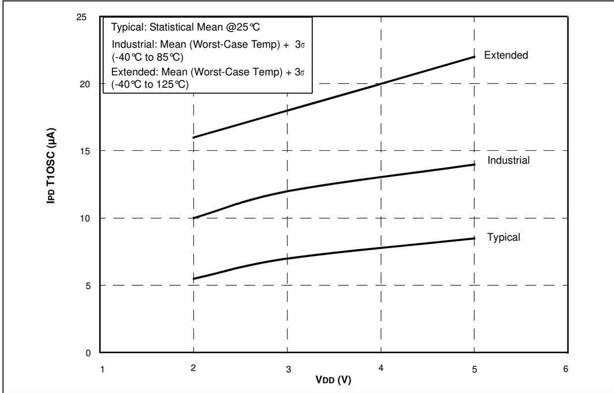
**FIGURE 17-17: PIC12F615/617 IPD A/D vs. VDD**
