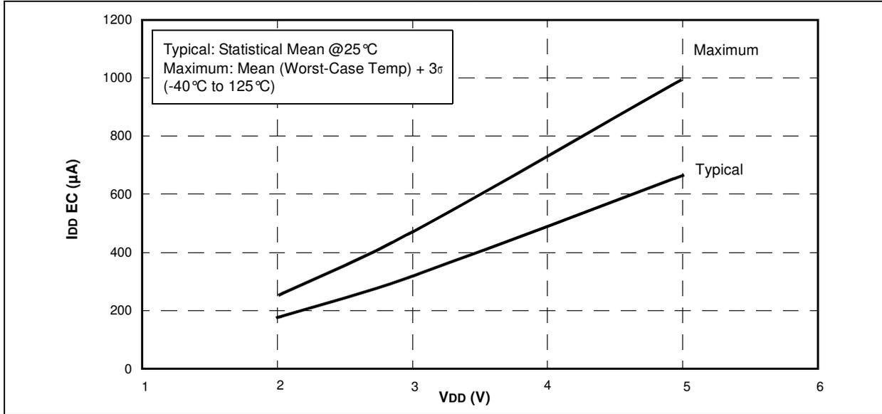
**FIGURE 17-4: PIC12F609/615/617 I<sub>DD XT</sub> (1 MHz) vs. V<sub>DD</sub>**
