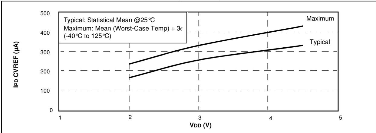
FIGURE 17-32: PIC12HV609/615 IPD T1OSC vs. VDD
