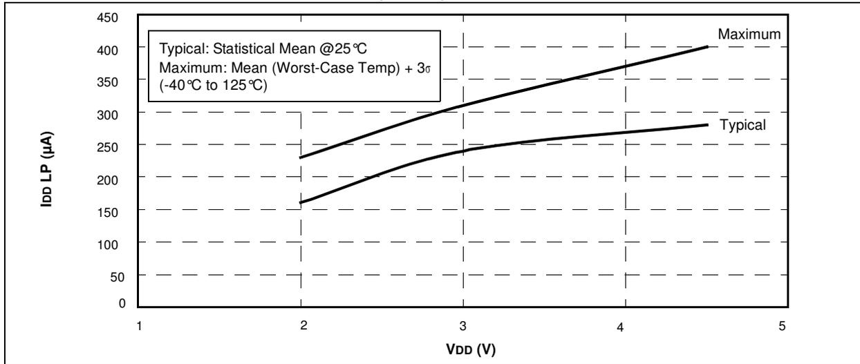
**FIGURE 17-19: PIC12HV609/615 I<sub>DD EC</sub> (1 MHz) vs. V<sub>DD</sub>**
