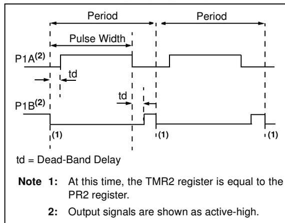
**FIGURE 11-9: EXAMPLE OF HALF-BRIDGE APPLICATIONS**
