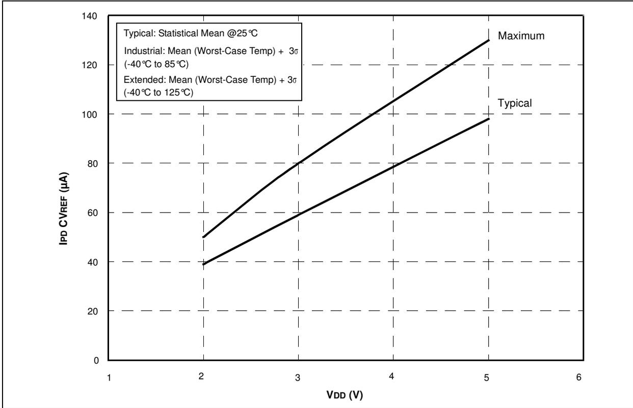
**FIGURE 17-15: PIC12F609/615/617 IPD CVREF (HI RANGE) vs. VDD**
