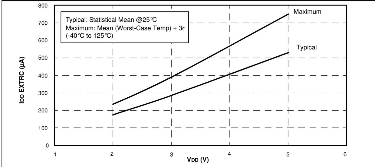
FIGURE 17-9: PIC12F609/615/617 I<sub>DD</sub> HS (20 MHz) vs. V<sub>DD</sub>
