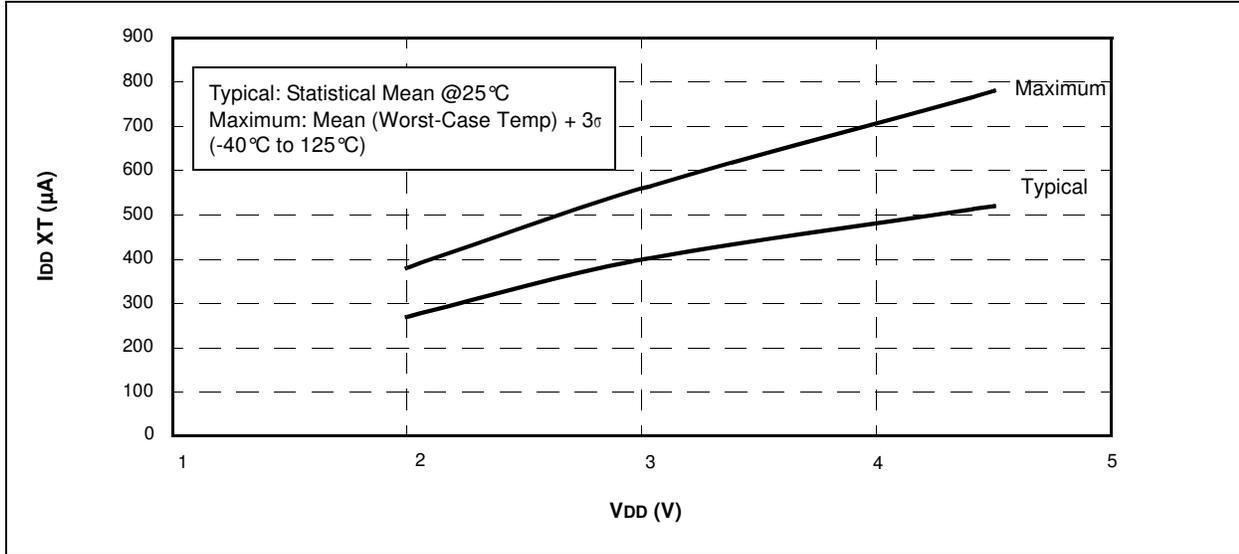
FIGURE 17-22: PIC12HV609/615 I<sub>DD XT</sub> (4 MHz) vs. V<sub>DD</sub>
