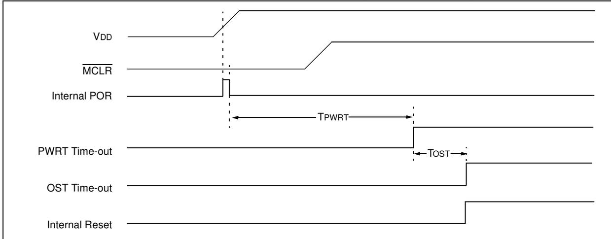
**FIGURE 12-5: TIME-OUT SEQUENCE ON POWER-UP (DELAYED  $\overline{\text{MCLR}}$ ): CASE 2**
