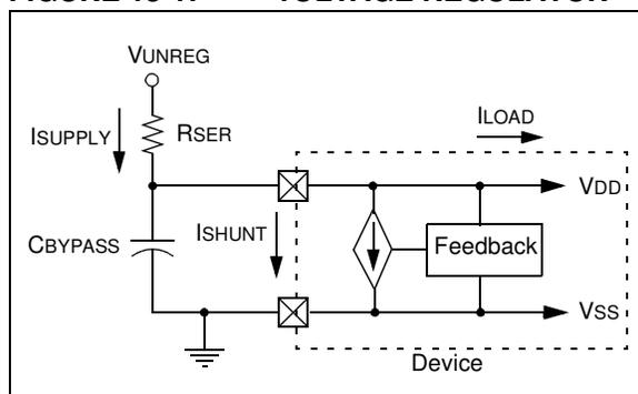
An external current limiting resistor, R<sub>SER</sub>, located between the unregulated supply, V<sub>UNREG</sub>, and the VDD pin, drops the difference in voltage between V<sub>UNREG</sub> and VDD. R<sub>SER</sub> must be between R<sub>MAX</sub> and R<sub>MIN</sub> as defined by Equation 13-1.
