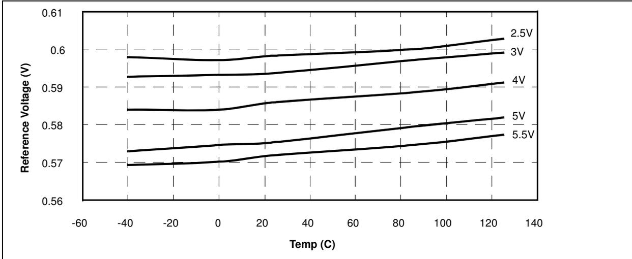
FIGURE 17-48: 1.2V REFERENCE VOLTAGE vs. TEMP (TYPICAL)
