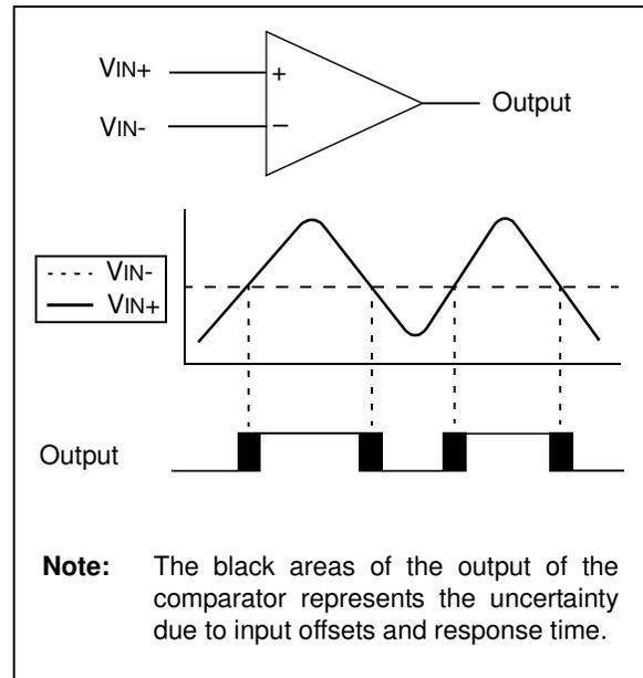
**FIGURE 9-2: COMPARATOR SIMPLIFIED BLOCK DIAGRAM**
