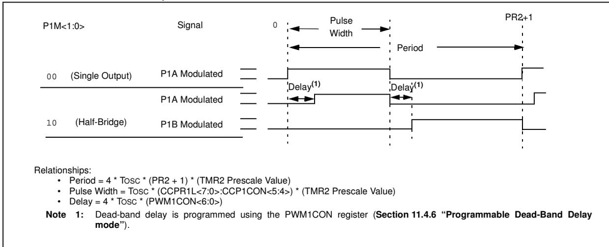
**FIGURE 11-7: EXAMPLE ENHANCED PWM OUTPUT RELATIONSHIPS (ACTIVE-LOW STATE)**
