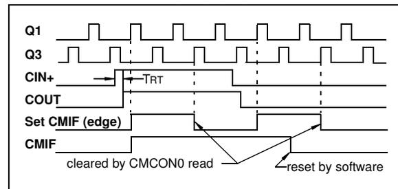
**Note 1:** If a change in the CMCON0 register (COUT) should occur when a read operation is being executed (start of the Q2 cycle), then the CMIF of the PIR1 register interrupt flag may not get set.
