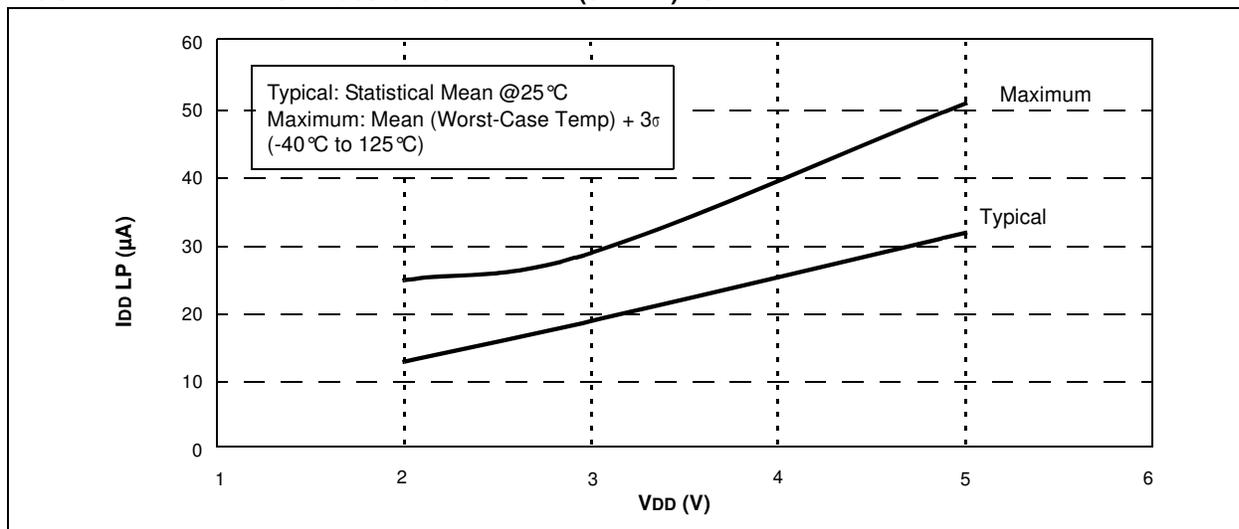
**FIGURE 17-2: PIC12F609/615/617 I<sub>DD EC</sub> (1 MHz) vs. V<sub>DD</sub>**
