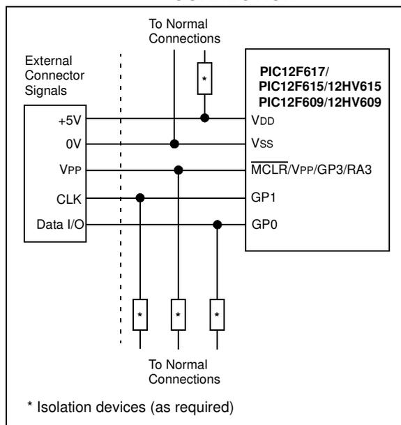
**Note:** To erase the device VDD must be above the Bulk Erase VDD minimum given in the *Memory Programming Specification* (DS41284)
