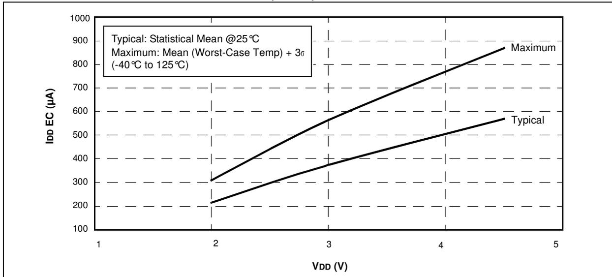
**FIGURE 17-20: PIC12HV609/615 I<sub>DD EC</sub> (4 MHz) vs. V<sub>DD</sub>**
