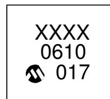
8-Lead DFN (4x4 mm) (for PIC12F609/615/HV609/615 devices only)
