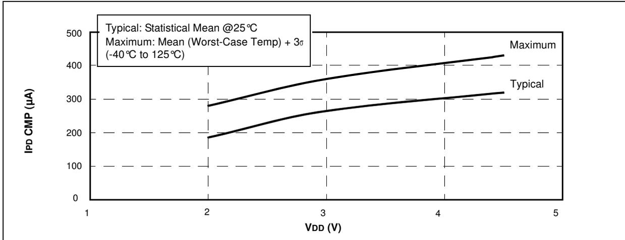
**FIGURE 17-28: PIC12HV609/615 IPD WDT vs. VDD**
