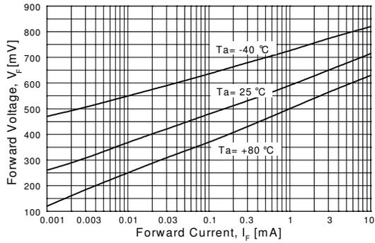
Figure 7. Forward Voltage vs Ambient Temperature
