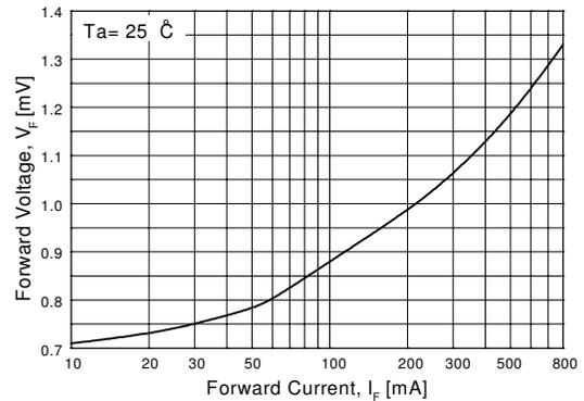
Figure 6. Forward Voltage vs Forward Current
