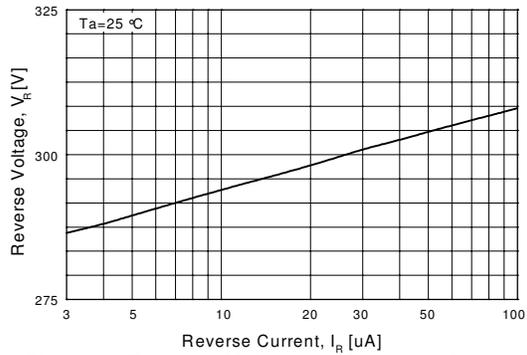
Figure 1. Reverse Voltage vs Reverse Current
