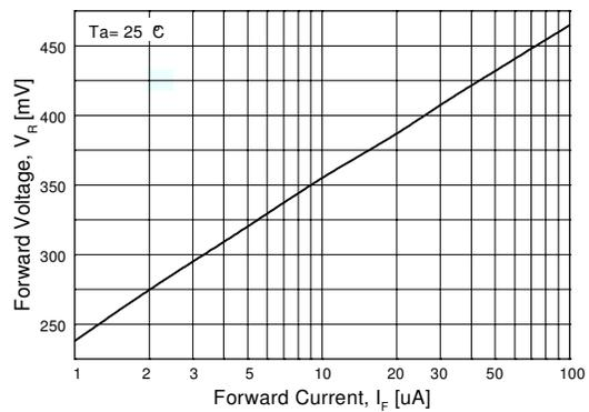
Figure 4. Forward Voltage vs Forward Current
