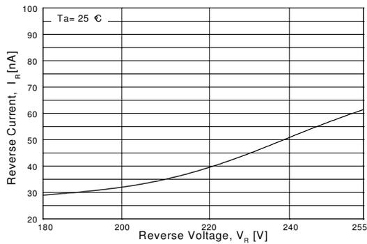
Figure 3. Reverse Current vs Reverse Voltage
