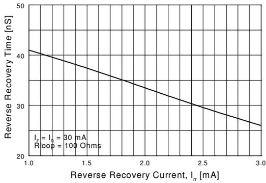
Figure 9. Reverse Recovery Time vs Reverse Recovery Current
