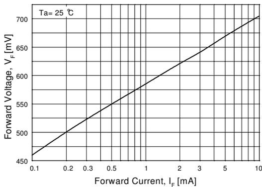
Figure 5. Forward Voltage vs Forward Current
