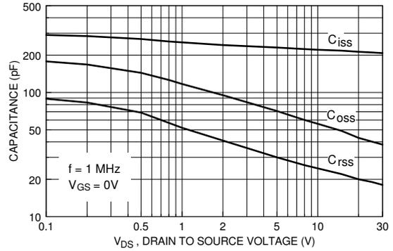
Figure 8. Capacitance Characteristics.
