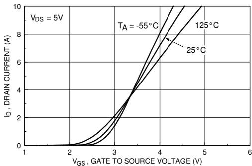
Figure 5. Transfer Characteristics.
