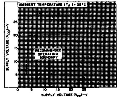
Fig. 10 – High-level supply voltage vs. low-level supply voltage.
