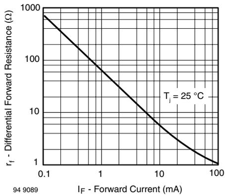
Figure 3. Differential Forward Resistance vs. Forward Current
