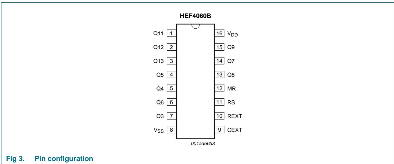
Fig 3. Pin configuration
