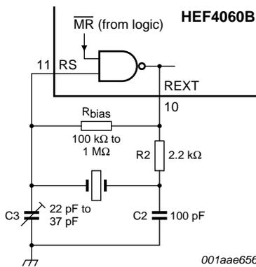
**Fig 7. External component connection for crystal oscillator**
