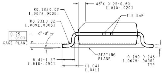
CONTROLLING DIMENSION IS MILLIMETER
