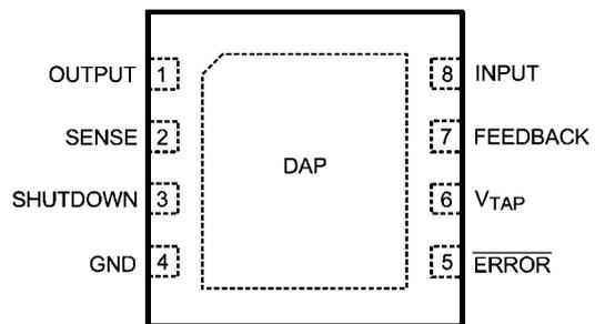
Connect DAP to GND at device pin 4.
