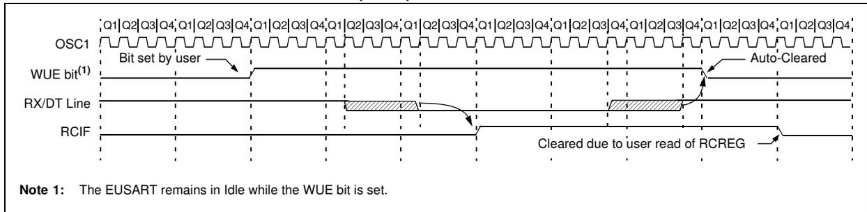
**FIGURE 18-9: AUTO-WAKE-UP BIT (WUE) TIMINGS DURING SLEEP**
