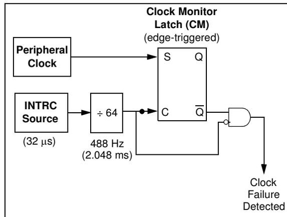
Clock failure is tested for on the falling edge of the sample clock. If a sample clock falling edge occurs while CM is still set, a clock failure has been detected (Figure 23-4). This causes the following:
