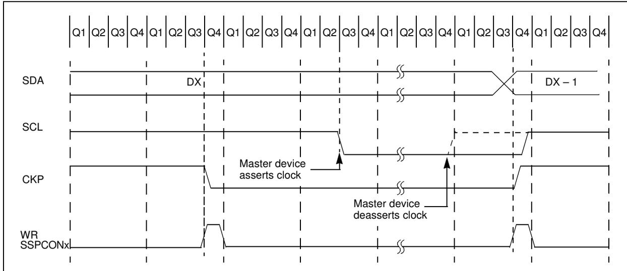
FIGURE 17-13: I<sup>2</sup>C™ SLAVE MODE TIMING WITH SEN = 1 (RECEPTION, 7-BIT ADDRESS)
