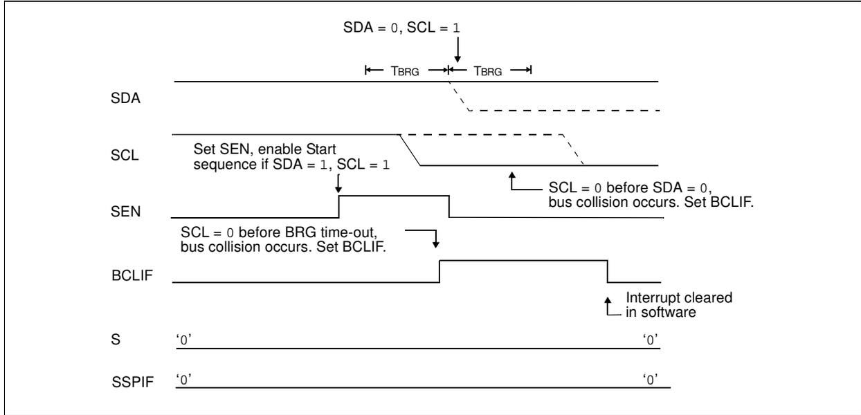
**FIGURE 17-28: BRG RESET DUE TO SDA ARBITRATION DURING START CONDITION**
