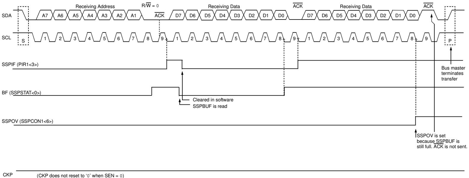
FIGURE 17-9: I<sup>2</sup>C™ SLAVE MODE TIMING (TRANSMISSION, 7-BIT ADDRESS)
