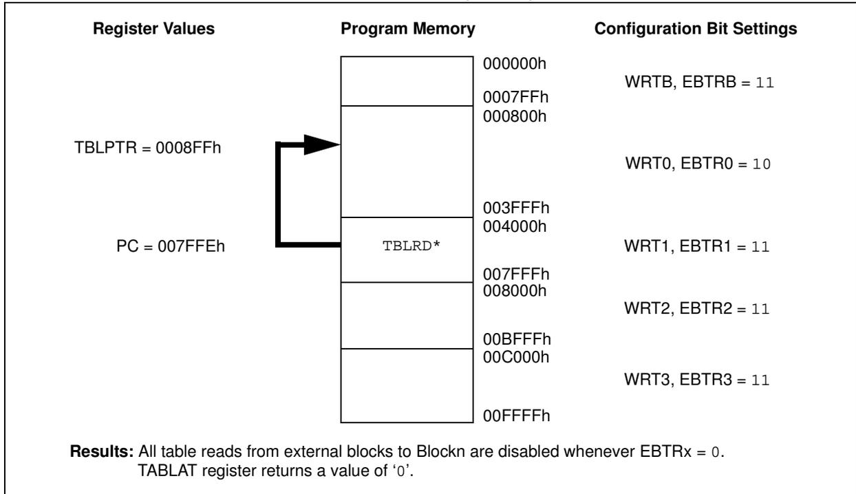
**FIGURE 23-8: EXTERNAL BLOCK TABLE READ (EBTRx) ALLOWED**
