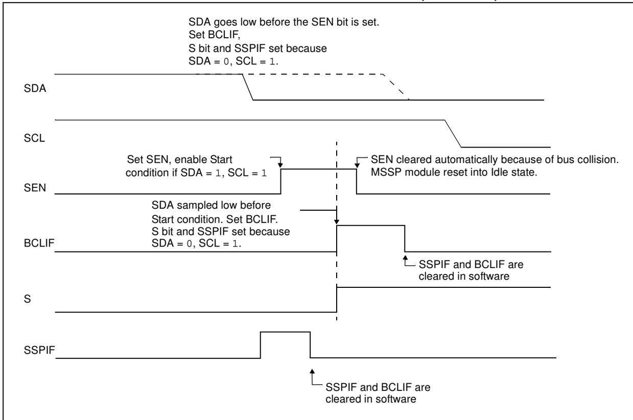
**FIGURE 17-27: BUS COLLISION DURING START CONDITION (SCL = 0)**
