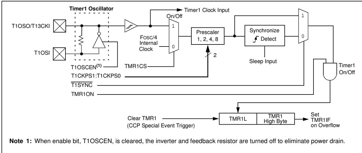
**FIGURE 12-2: TIMER1 BLOCK DIAGRAM (16-BIT READ/WRITE MODE)**
