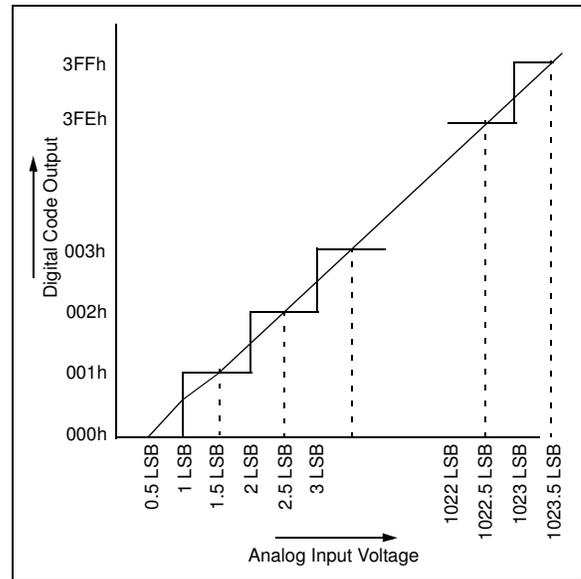
**FIGURE 19-3: ANALOG INPUT MODEL**
