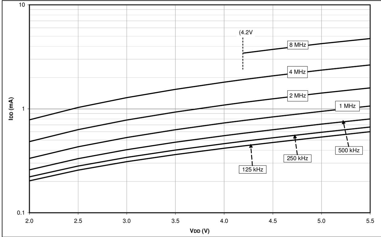
FIGURE 27-12: MAXIMUM  $I_{DD}$  ACROSS  $V_{DD}$  (RC\_RUN MODE, 85°C)
