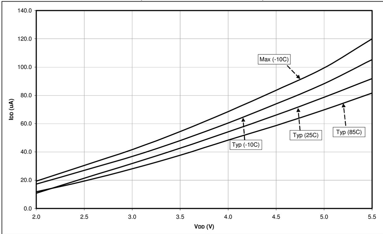
**FIGURE 27-18: TYPICAL AND MAXIMUM SEC\_IDLE CURRENT vs. V<sub>DD</sub> ACROSS TEMPERATURE (T1OSC IN LOW-POWER MODE)**
