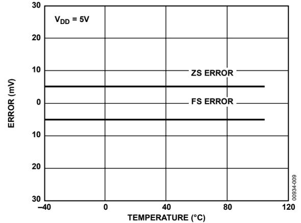
Figure 9. Zero-Scale Error and Full-Scale Error vs. Temperature
