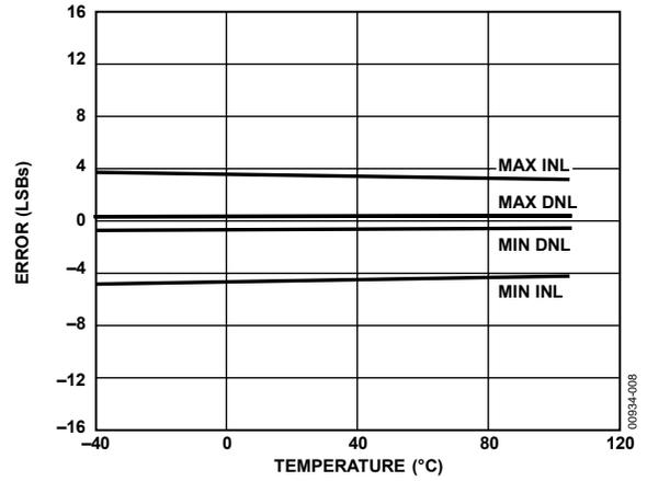
Figure 8. INL Error and DNL Error vs. Temperature
