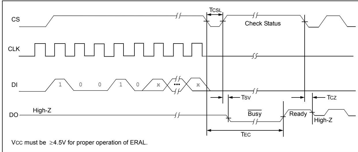
FIGURE 2-4: ERAL TIMING FOR 93C DEVICES
