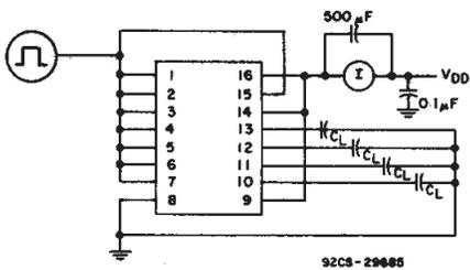
Fig. 9 — Dynamic power dissipation test circuit.
