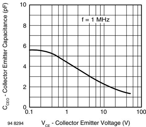
Fig. 6 - Collector Emitter Capacitance vs. Collector Emitter Voltage
