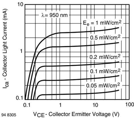
Fig. 5 - Collector Light Current vs. Collector Emitter Voltage
