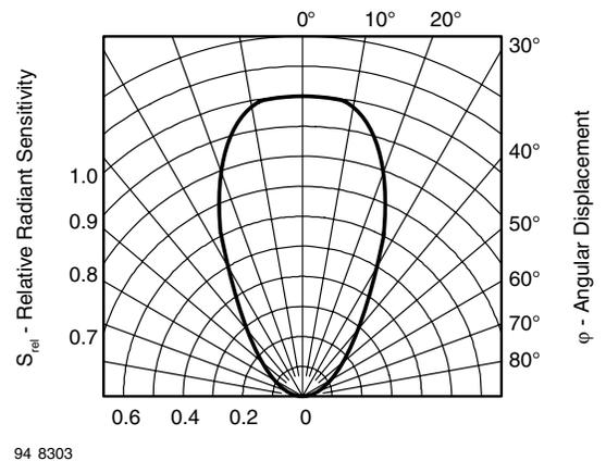
Fig. 9 - Relative Radiant Sensitivity vs. Angular Displacement
