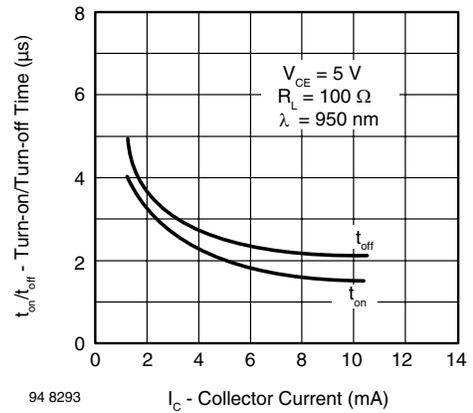
Fig. 7 - Turn-on/Turn-off Time vs. Collector Current
