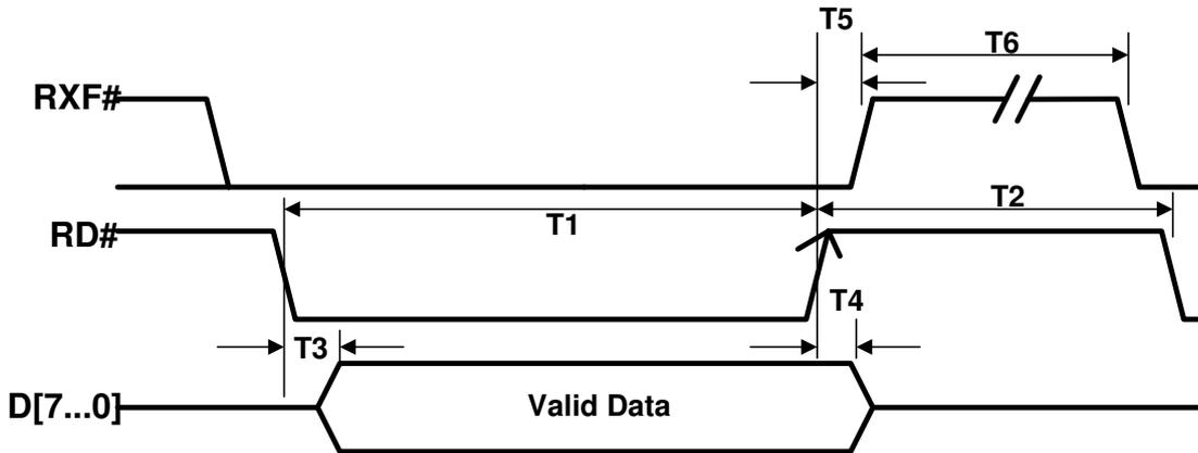
Figure 4.5 FT245 asynchronous FIFO Interface READ Signal Waveforms
