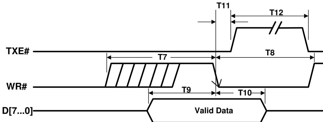
Figure 4.6 FT245 asynchronous FIFO Interface WRITE Signal Waveforms
