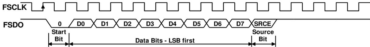
**Figure 4.14 Fast Opto-Isolated Serial Interface Output Data**
