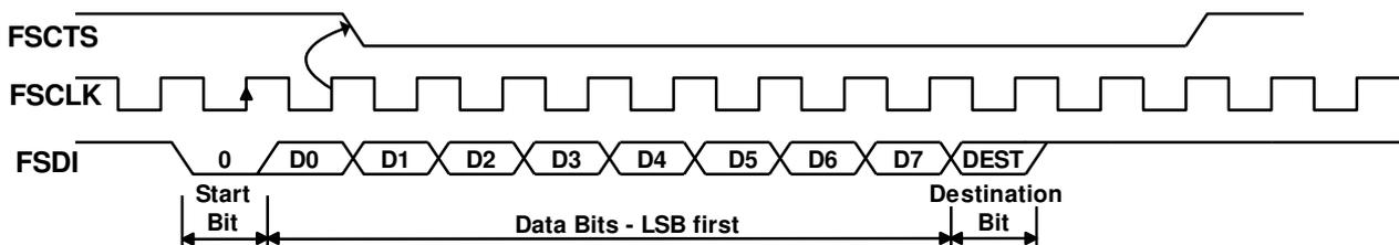
**Figure 4.15 Fast Opto-Isolated Serial Interface Input Data**
