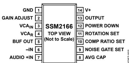
Figure 3. Pin Configuration
