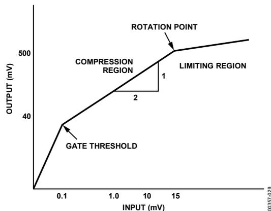
Figure 30. Transfer Characteristic
