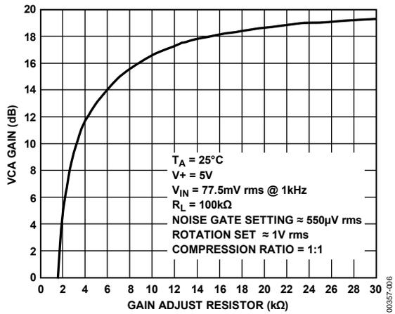
Figure 6. VCA Gain vs.  $R_{GAIN}$  (Pin 2 to GND)
