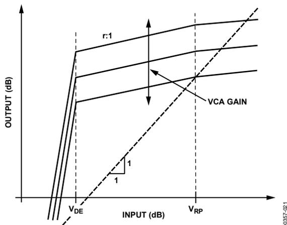
Figure 22. Effect of Varying the VCA Gain Setting
