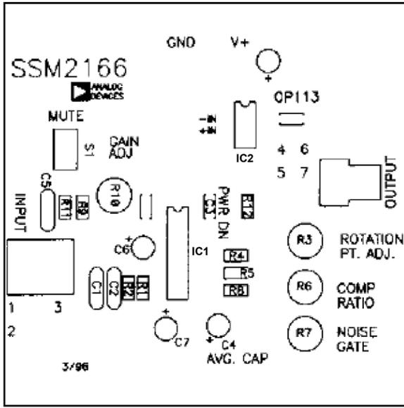
Figure 27. Evaluation Board Topside Silkscreen (Not to Scale)
