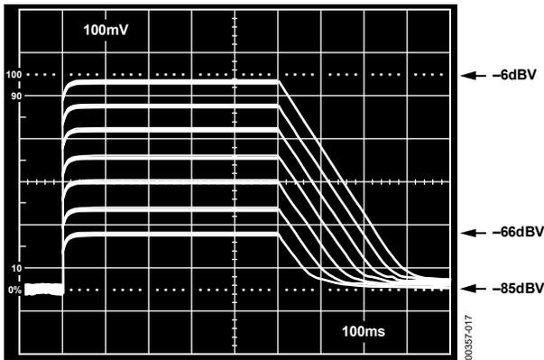
Figure 17. RMS Level Detector Performance with  $C_{AVG} = 2.2 \mu\text{F}$
