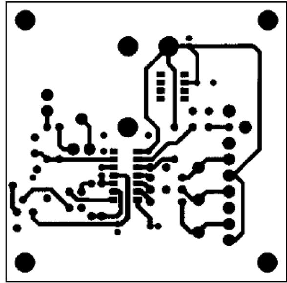
Figure 29. Evaluation Board Backside Metallization (Not to Scale)
