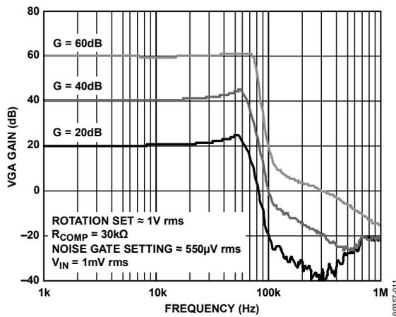
Figure 11. VCA Gain Bandwidth Curves vs. Frequency
