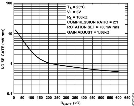
Figure 5. Noise Gate vs.  $R_{GATE}$  (Pin 9 to  $V_+$ )
