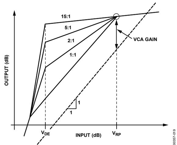
Figure 20. Effect of Varying the Compression Ratio
