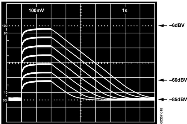
Figure 18. RMS Level Detector Performance with  $C_{AVG} = 22 \mu\text{F}$
