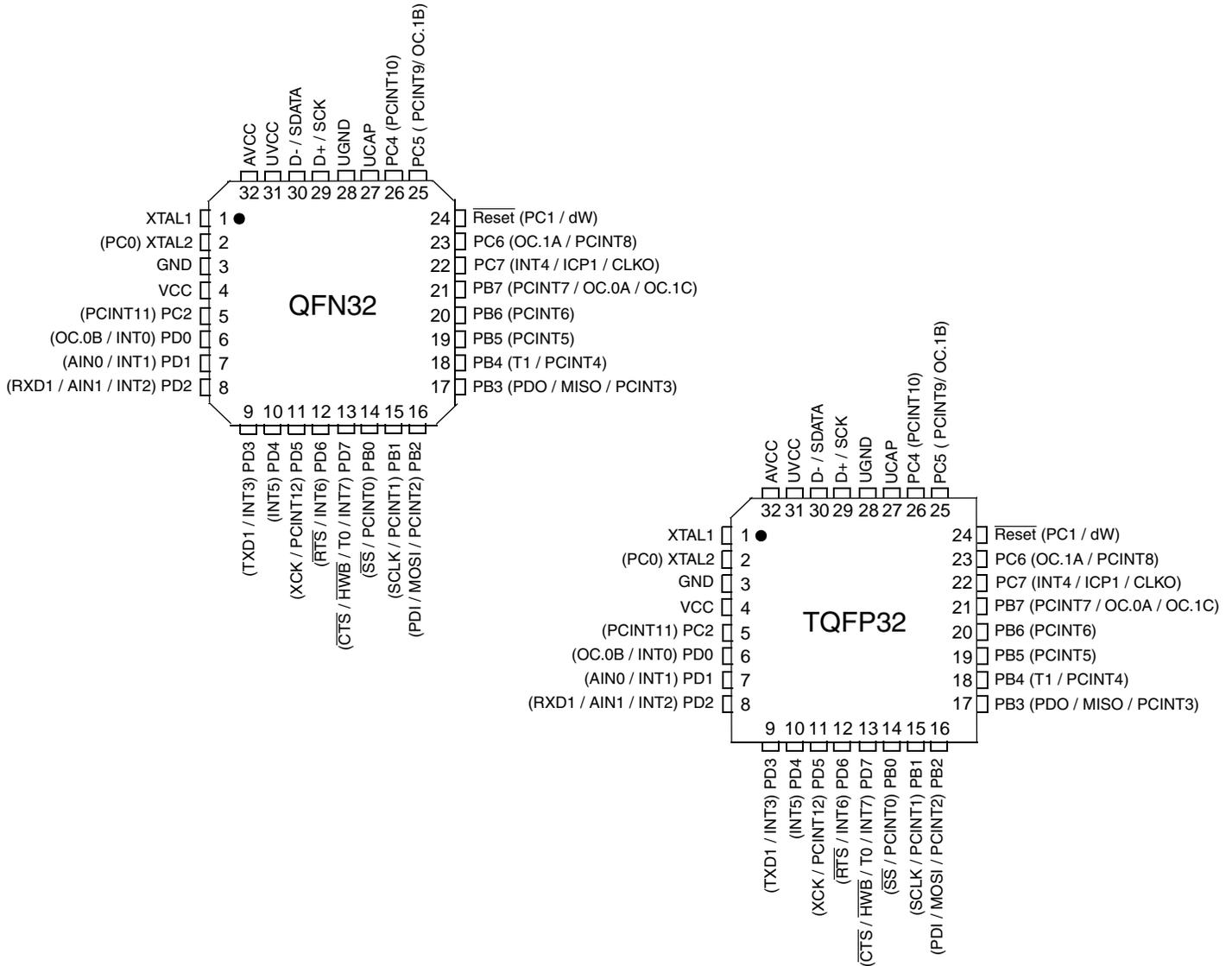
Note: The large center pad underneath the QFN packages is made of metal and must be connected to GND. It should be soldered or glued to the board to ensure good mechanical stability. If the center pad is left unconnected, the package might loosen from the board.
