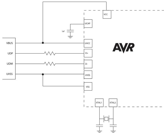
Figure 19-4. Typical Bus powered application with 3V I/O
