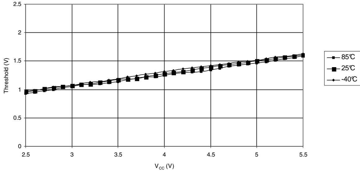
**Figure 27-4.** Input High Voltage vs. V<sub>CC</sub>, MOSI/MISO I/Os
