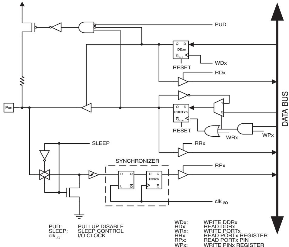
Note: 1. WRx, WPx, WDx, RRx, RPx, and RDx are common to all pins within the same port. clk<sub>I/O</sub>, SLEEP, and PUD are common to all ports.
