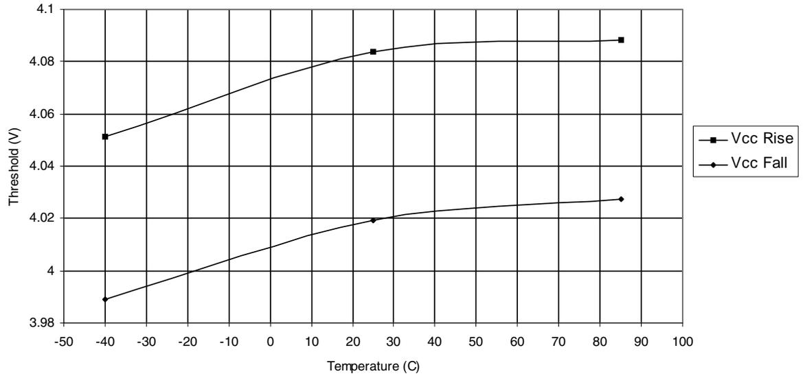
**Figure 27-30. BOD Voltage (4.3V level) vs. Temperature**
