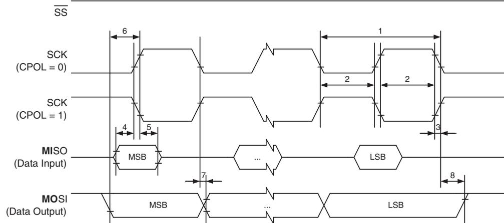
**Table 26-3.** SPI Interface Timing Requirements (Slave Mode)
