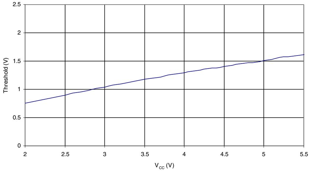
**Figure 27-2.** Input High Voltage vs. V<sub>CC</sub>, all I/Os excluding DP/DM and MOSI/MISO
