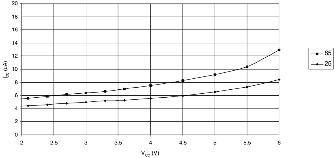
Figure 27-12. Power-down Supply Current vs. V<sub>CC</sub>, with BOD Disabled, WDT Enabled, Regulator Disabled
