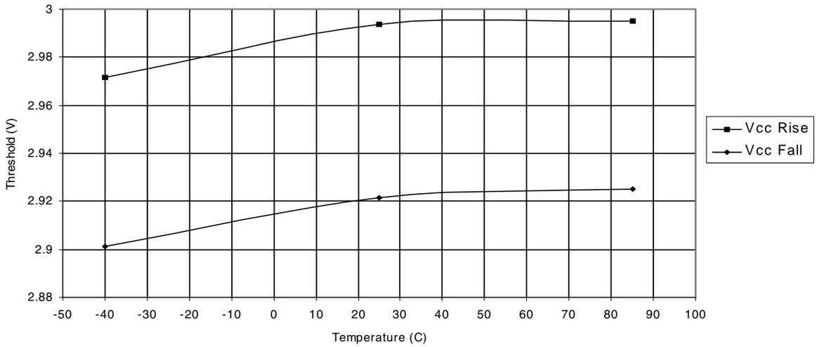
**Figure 27-26. BOD Voltage (3.0V level) vs. Temperature**
