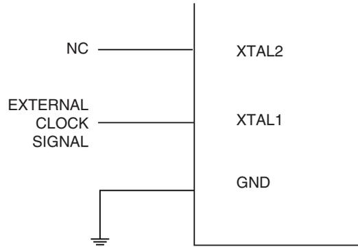
When this clock source is selected, start-up times are determined by the SUT Fuses as shown in [Table 6-8](#).
