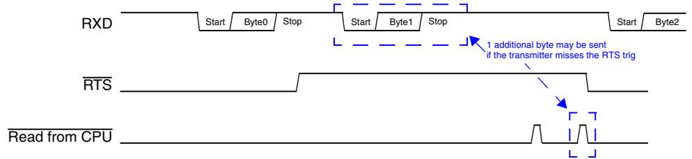
$\overline{\text{RTS}}$  will rise at 2/3 of the last received stop bit if the receive fifo is full.
