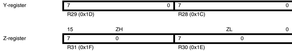
In the different addressing modes these address registers have functions as fixed displacement, automatic increment, and automatic decrement (see the instruction set reference for details).
