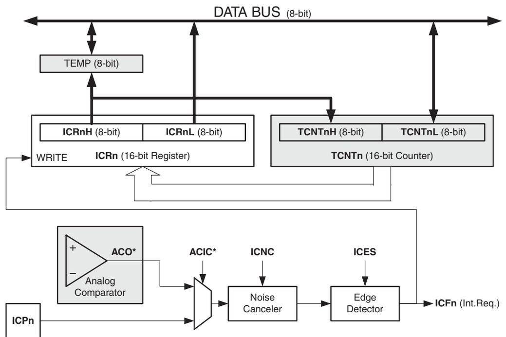
Note: The Analog Comparator Output (ACO) can only trigger the Timer/Counter1 ICP – not Timer/Counter3, 4 or 5.
