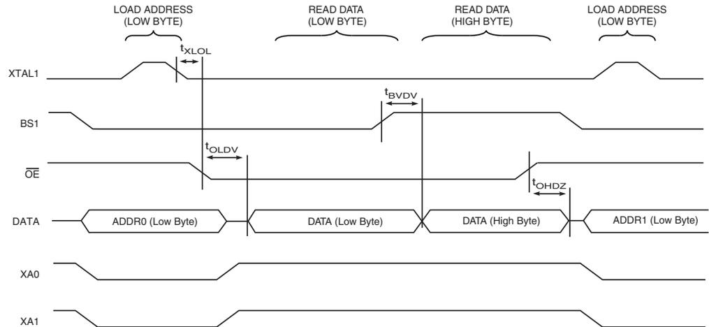
Note: 1. The timing requirements shown in Figure 25-7 (i.e.,  $t_{DVXH}$ ,  $t_{XHXL}$ , and  $t_{XLDX}$ ) also apply to reading operation.
