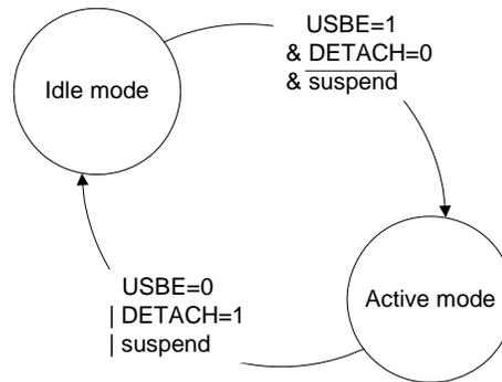
The SUSPI flag indicated that a suspend state has been detected on the USB bus. This flag automatically put the USB pad in Idle. The detection of a non-idle event sets the WAKEUPI flag and wakes-up the USB pad.
