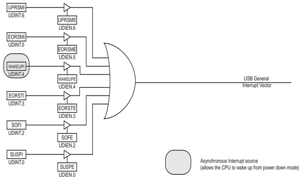
Each of these interrupts are time-relative events that will be detected only if the USB clock is enabled (FRZCLK bit cleared), except for the WAKEUP interrupt that will trigger each time a state change is detected on the data lines.
