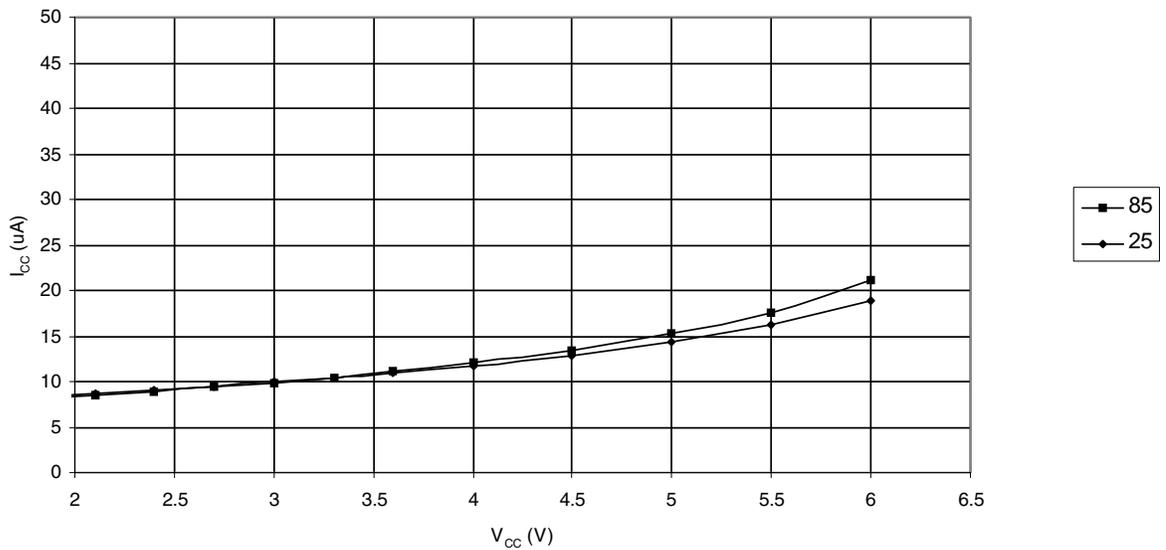
**Figure 27-13.** Power-down Supply Current vs.  $V_{CC}$ , with BOD Enabled, Watchdog Disabled
