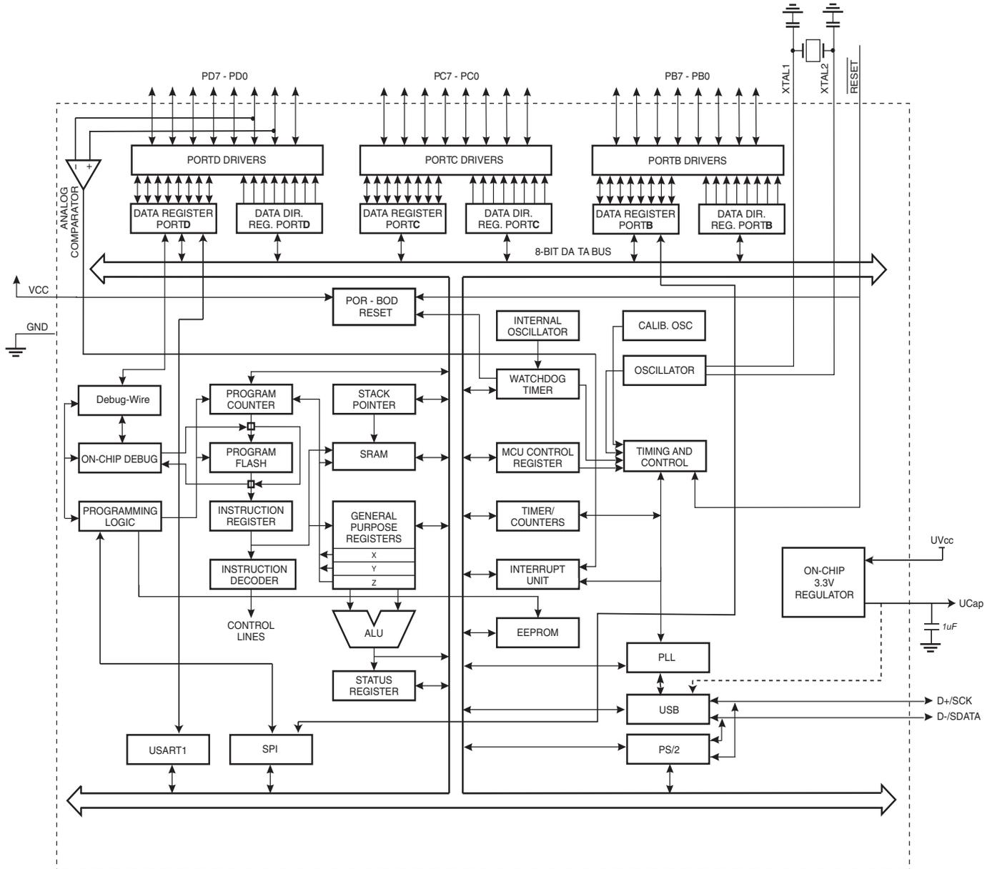
The AVR core combines a rich instruction set with 32 general purpose working registers. All the 32 registers are directly connected to the Arithmetic Logic Unit (ALU), allowing two independent registers to be accessed in one single instruction executed in one clock cycle. The resulting
