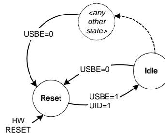
The reset state of the Device controller is:
