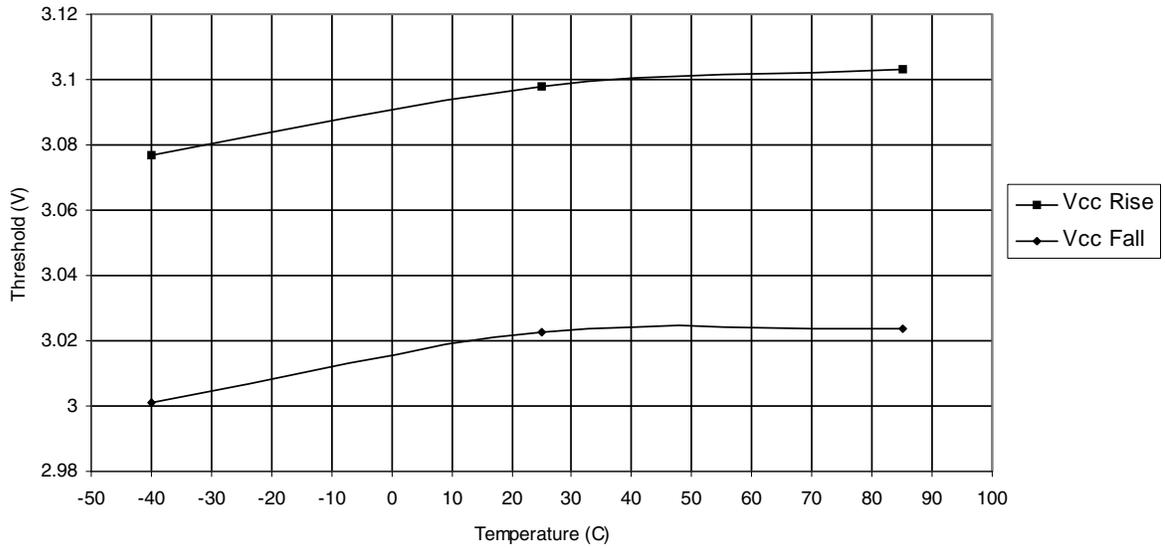
**Figure 27-27. BOD Voltage (3.5V level) vs. Temperature**
