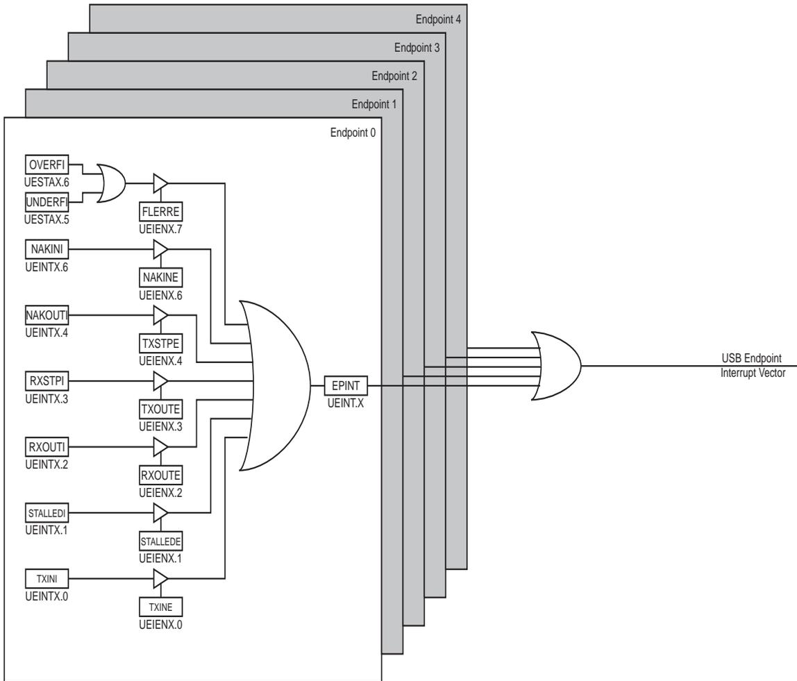
Each endpoint has 8 interrupts sources associated with flags, and each source can be enabled or not to trigger the corresponding endpoint interrupt.
