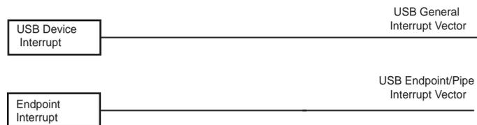
The macro distinguishes between USB General events in opposition with USB Endpoints events that are relevant with data transfers relatives to each endpoint.
