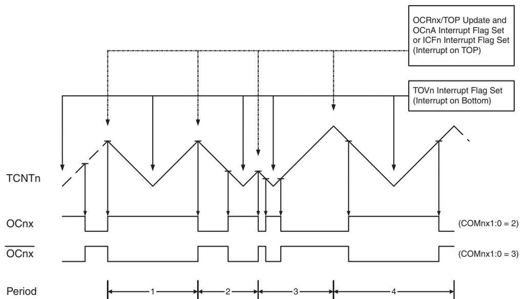
The Timer/Counter Overflow Flag (TOVn) is set each time the counter reaches BOTTOM. When either OCRnA or ICRn is used for defining the TOP value, the OCNxA or ICFn Flag is set accordingly at the same timer clock cycle as the OCRnx Registers are updated with the double buffer value (at TOP). The Interrupt Flags can be used to generate an interrupt each time the counter reaches the TOP or BOTTOM value.
