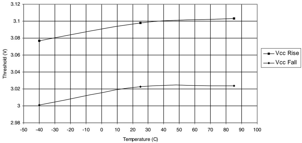
Figure 27-28. BOD Voltage (3.6V level) vs. Temperature
