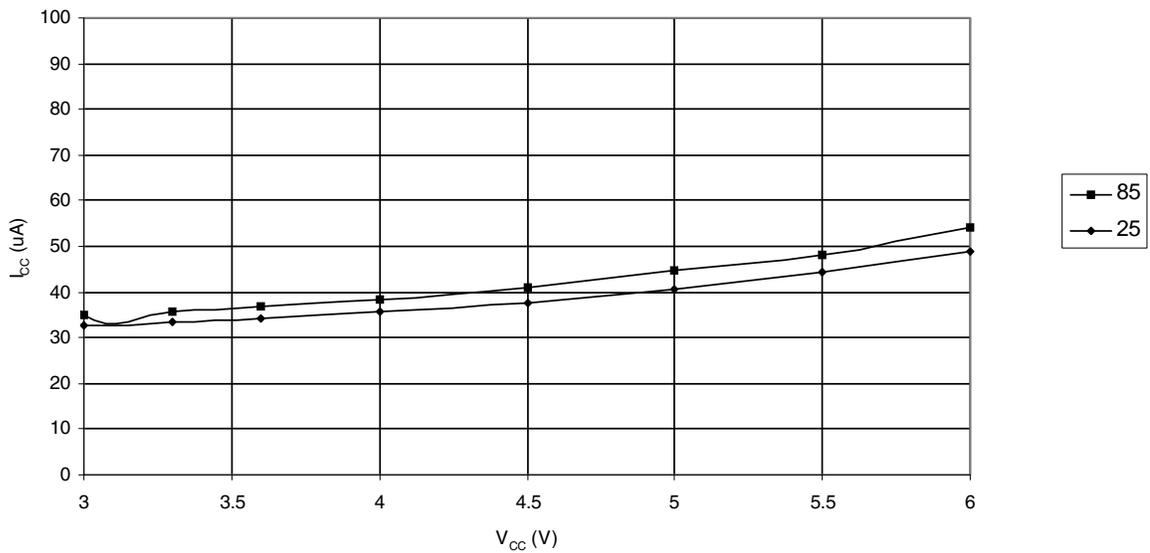
Figure 27-15. Power-down Supply Current vs. Vcc, with BOD Enabled, Regulator Enabled
