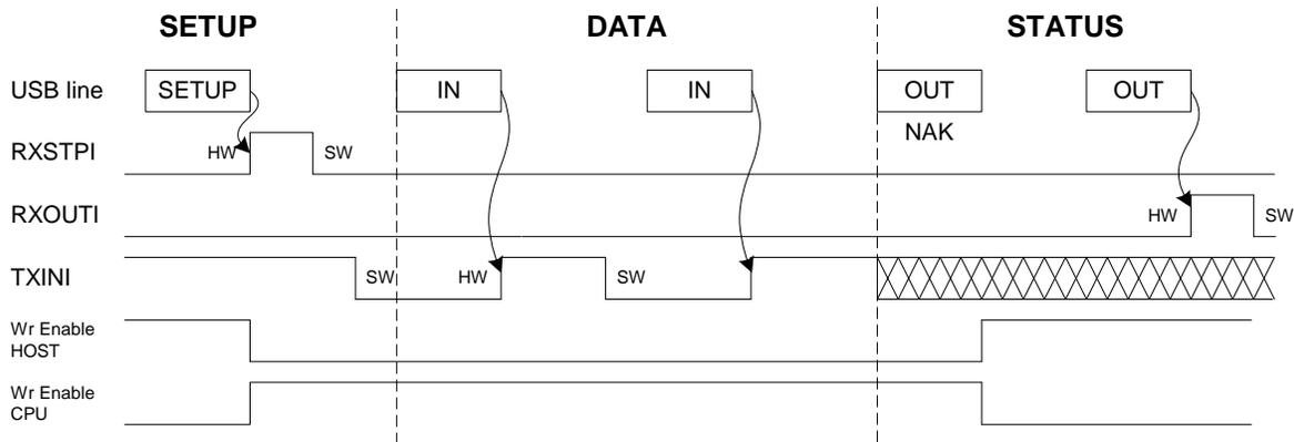
A NAK handshake is always generated at the first status stage command.
