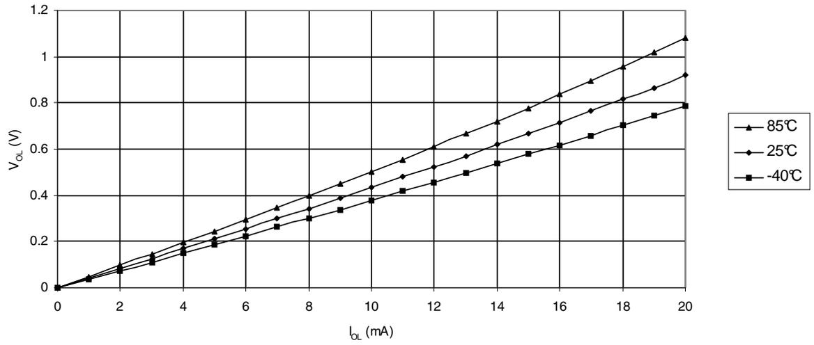
Figure 27-8. Output High Voltage vs. Output Current, all I/Os excluding DP/DM, Vcc=3V
