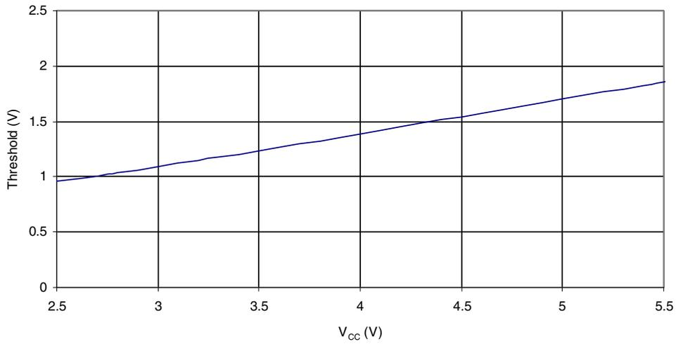
**Figure 27-3.** Input Low Voltage vs. V<sub>CC</sub> for MOSI/MISO I/Os
