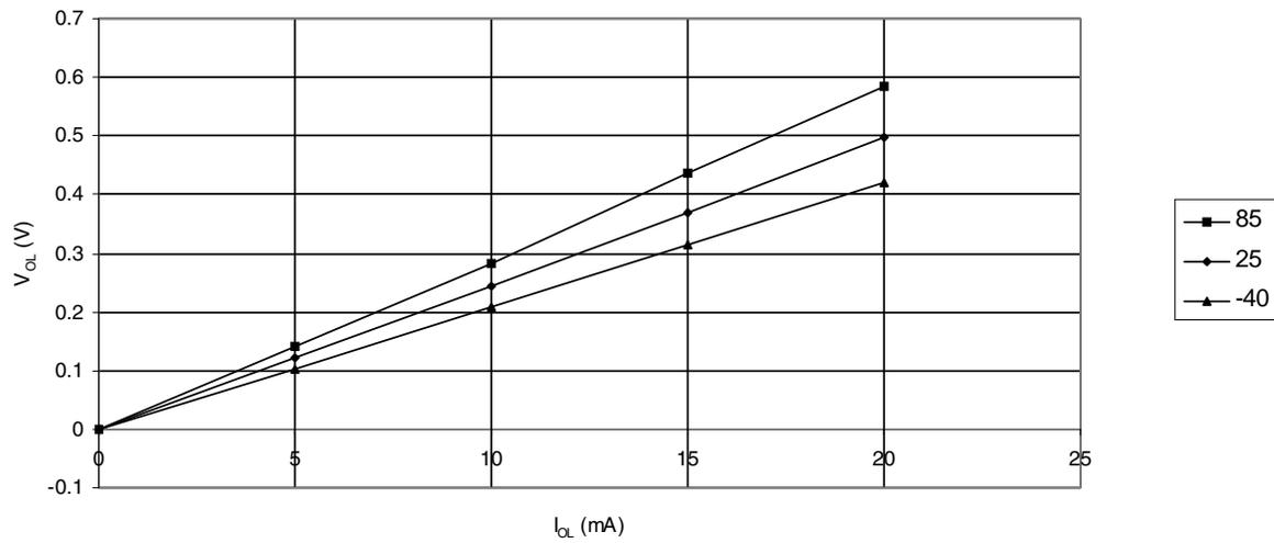
**Figure 27-7.** Output Low Voltage vs. Output Current, PS2 I/Os,  $V_{CC}=5V$
