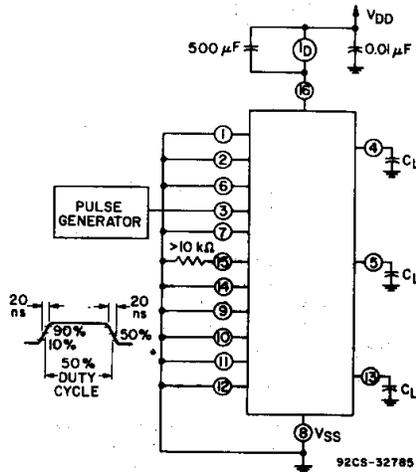
Fig. 20—Dynamic power dissipation test circuit and waveform.
