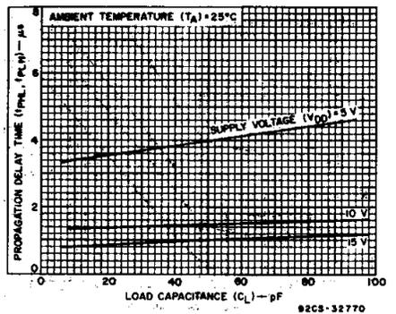
**Fig. 9—Typical propagation delay time as a function of load capacitance (CLOCK to Q<sub>16</sub>, 8-BYPASS high).**
