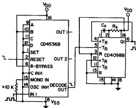
Fig. 30—Application showing use of CD4098B and CD4536B to get decode pulse 8 clock pulses after Reset pulse.
