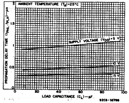
**Fig. 7—Typical propagation delay time as a function of load capacitance (CLOCK to Q<sub>1</sub>, 8-BYPASS high).**
