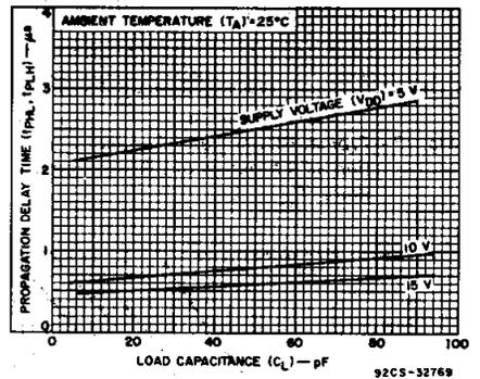
**Fig. 8—Typical propagation delay time as a function of load capacitance (CLOCK to Q<sub>1</sub>, 8-BYPASS low).**
