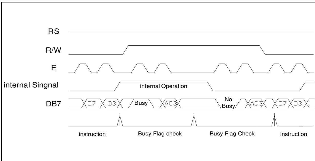
Figure 7.0 Example of 4-bit bus mode timing diagram
