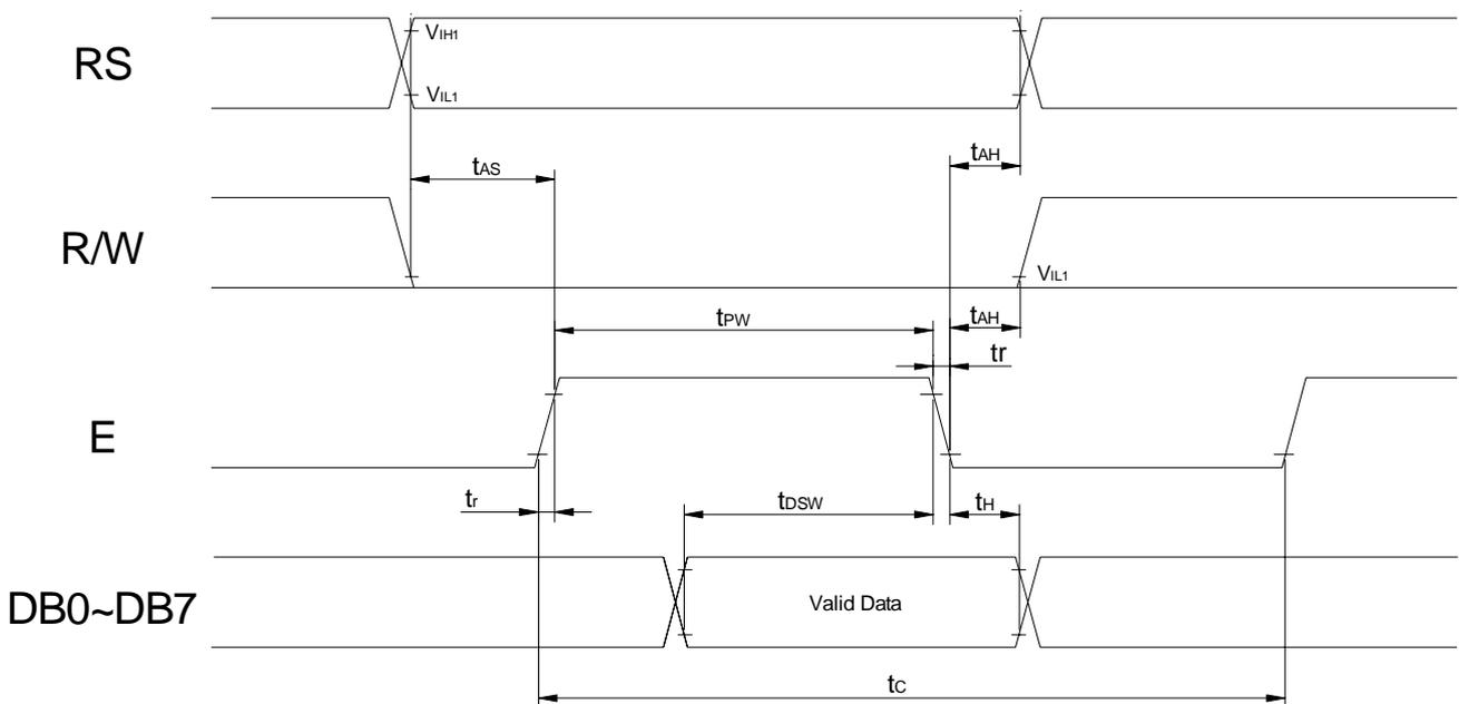
12-2-2 Read mode (reading data from module to MPU )
