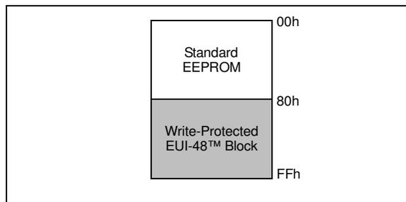
The 6-byte EUI-48 node address value is stored in array locations 0xFA through 0xFF, as shown in Figure 3-2. The first 3 bytes are the Organizationally Unique Identifier (OUI) assigned to Microchip by the IEEE Registration Authority. The remaining 3 bytes are the Extension Identifier, and are generated by Microchip to ensure a globally-unique, 48-bit value.
