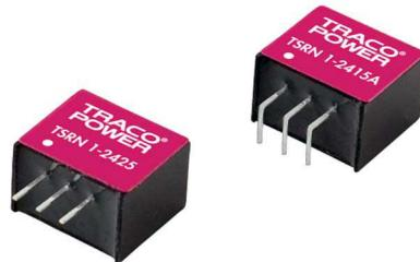
The new TSRN-1 series step-down switching regulators are drop-in replacement for inefficient 78xx linear regulators. A high efficiency up to 95 % allows full load operation up to  $+70^{\circ}\text{C}$  ( $+85^{\circ}\text{C}$  with derating) ambient temperature without the need of any heat-sink or forced air cooling.
