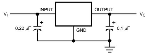
**Note:** Bypass capacitors are recommended for optimum stability and transient response, and should be located as close as possible to the regulator.
