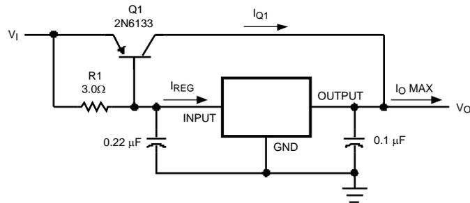
$$\beta(Q1) \geq \frac{I_{O\ Max}}{I_{REG\ Max}}$$
