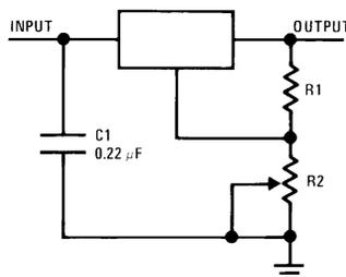
$$V_{\text{OUT}} = 5V + (5V/R1 + I_Q) R2 \quad 5V/R1 > 3 I_Q$$
