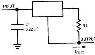
$$I_{OUT} = \frac{V_{2-3}}{R_1} + I_Q$$
