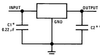
\*Required if the regulator is located far from the power supply filter.
