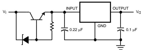
Figure 18. High Current Voltage Regulator
