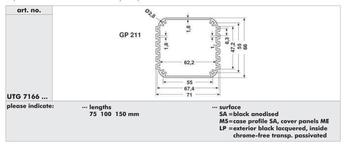
profiles in meter lengths 1000 mm → M 24
