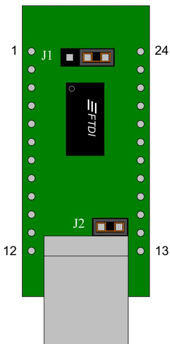
Figure 4 - Bus Powered Configuration
