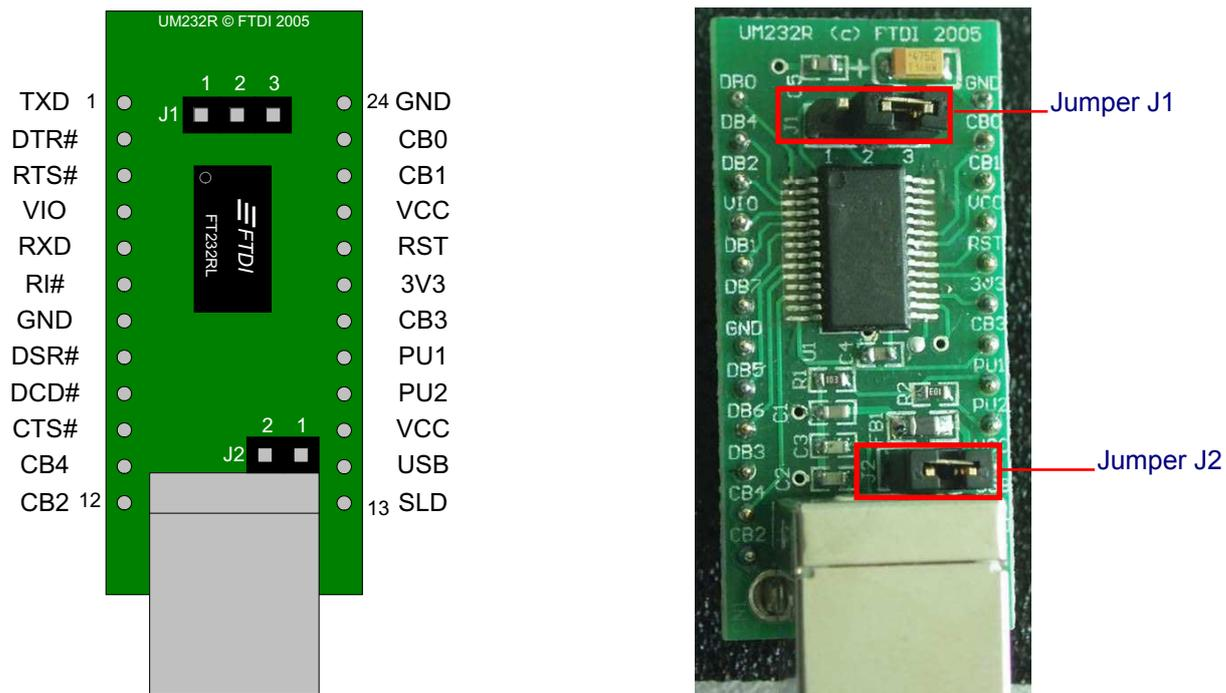
Figure 2 - Module Pin Out and Jumper locations.
