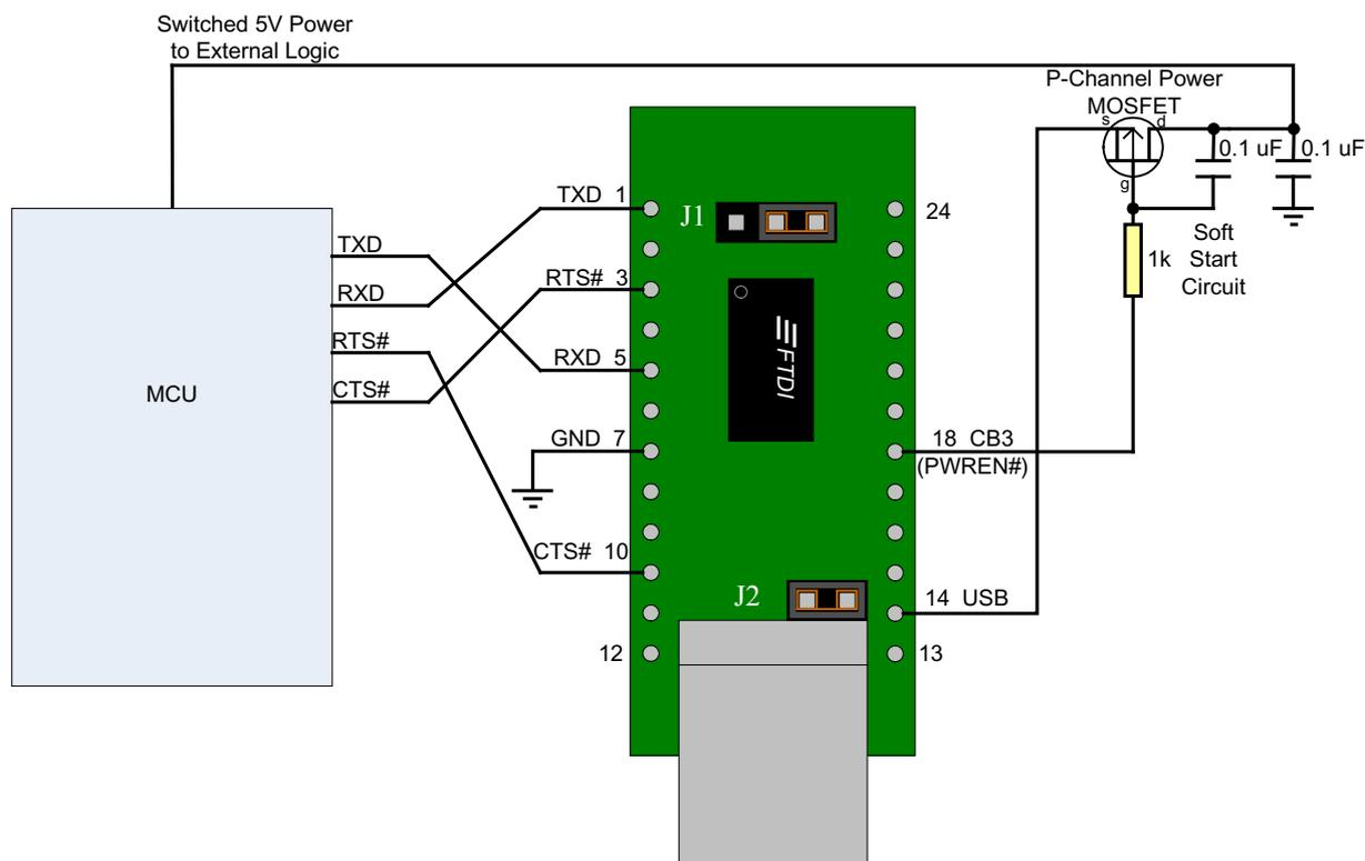
Figure 6 - Bus Powered with Power Switching Configuration
