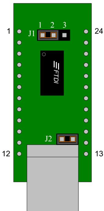
Figure 7 - USB Bus Powered 3.3V Logic Drive
