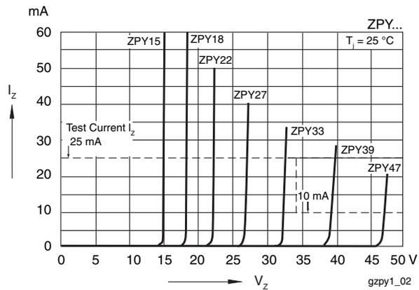
Fig. 8 - Breakdown Characteristics
