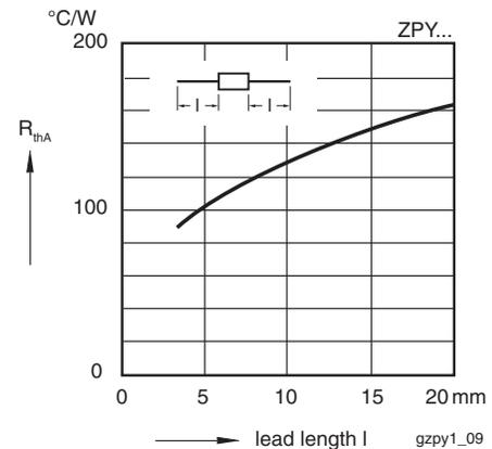
Fig. 6 - Thermal Resistance vs. Lead Length
