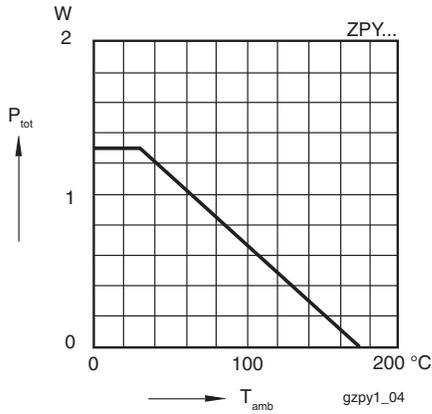
Fig. 1 - Admissible Power Dissipation vs. Ambient Temperature
