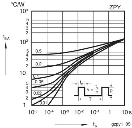
Fig. 2 - Pulse Thermal Resistance vs. Pulse Duration
