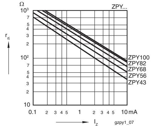
Fig. 4 - Dynamic Resistance vs. Zener Current
