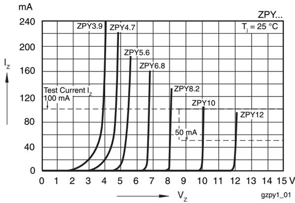
Fig. 7 - Breakdown Characteristics
