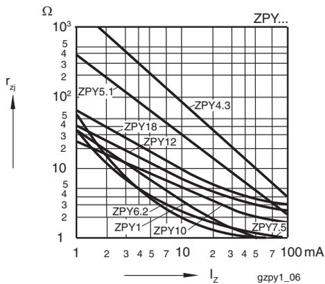
Fig. 3 - Dynamic Resistance vs. Zener Current
