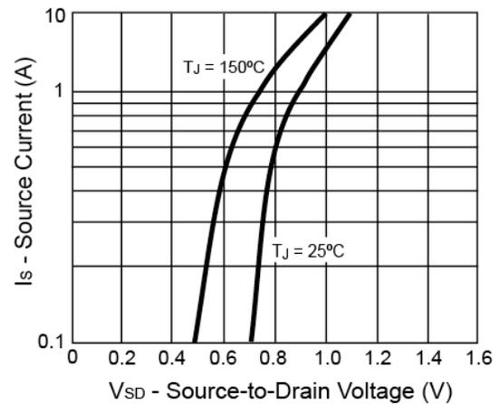
**Electrical Characteristics Curve** ( $T_a = 25^\circ\text{C}$ , unless otherwise noted)
