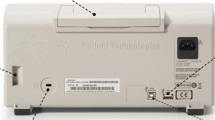
Two USB host ports facilitate saving data to a USB flash drive and enable quick firmware updates
