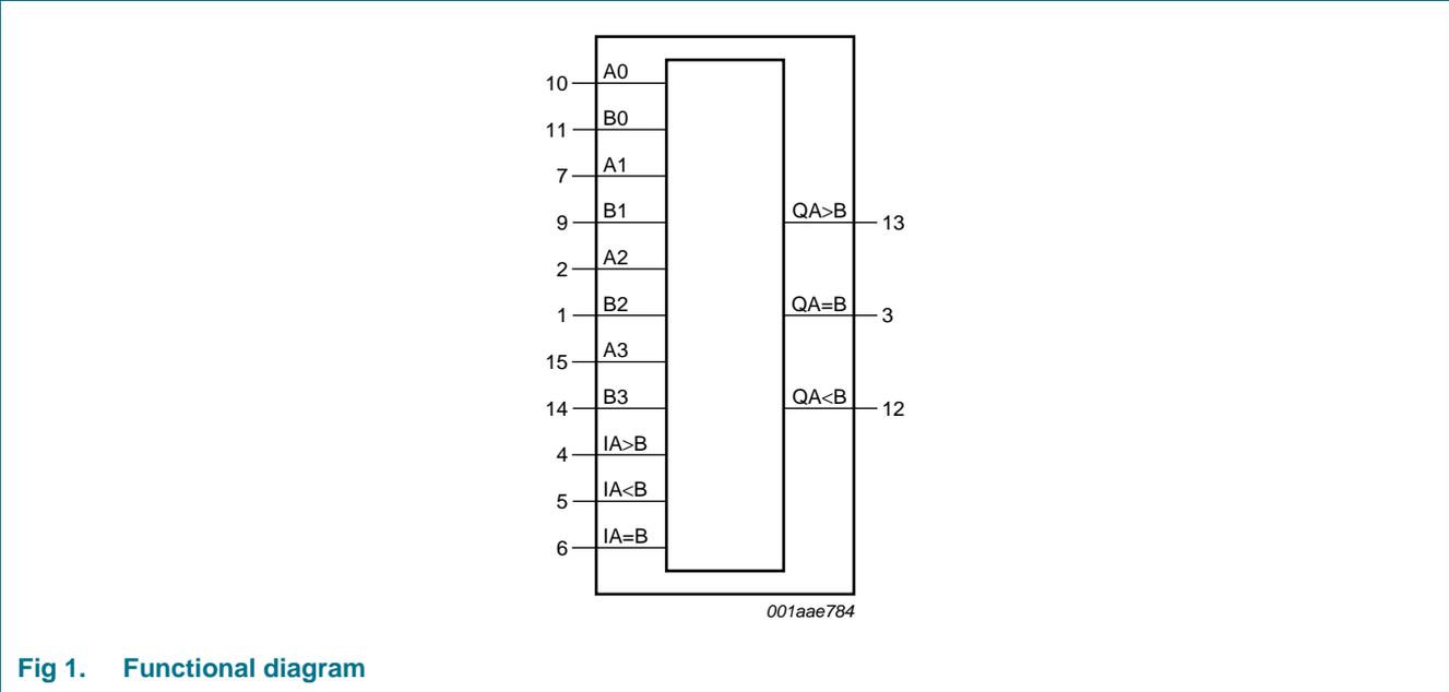
Fig 1. Functional diagram
