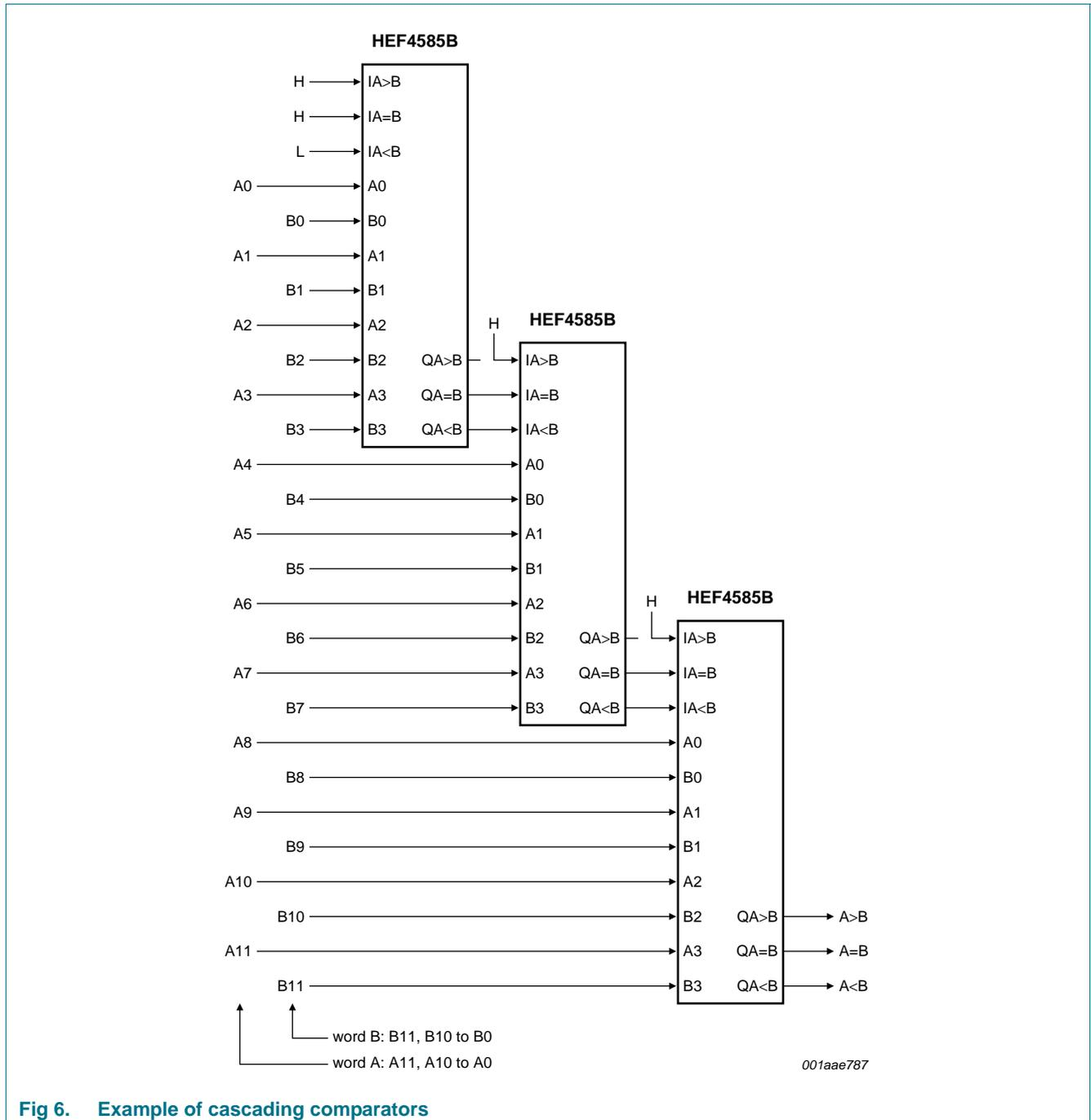
Fig 6. Example of cascading comparators
