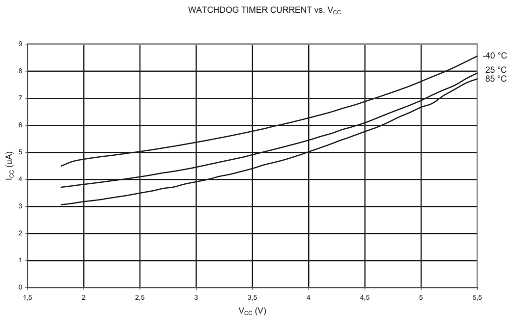
Figure 17-50. Watchdog Timer Current vs. V_{CC}
