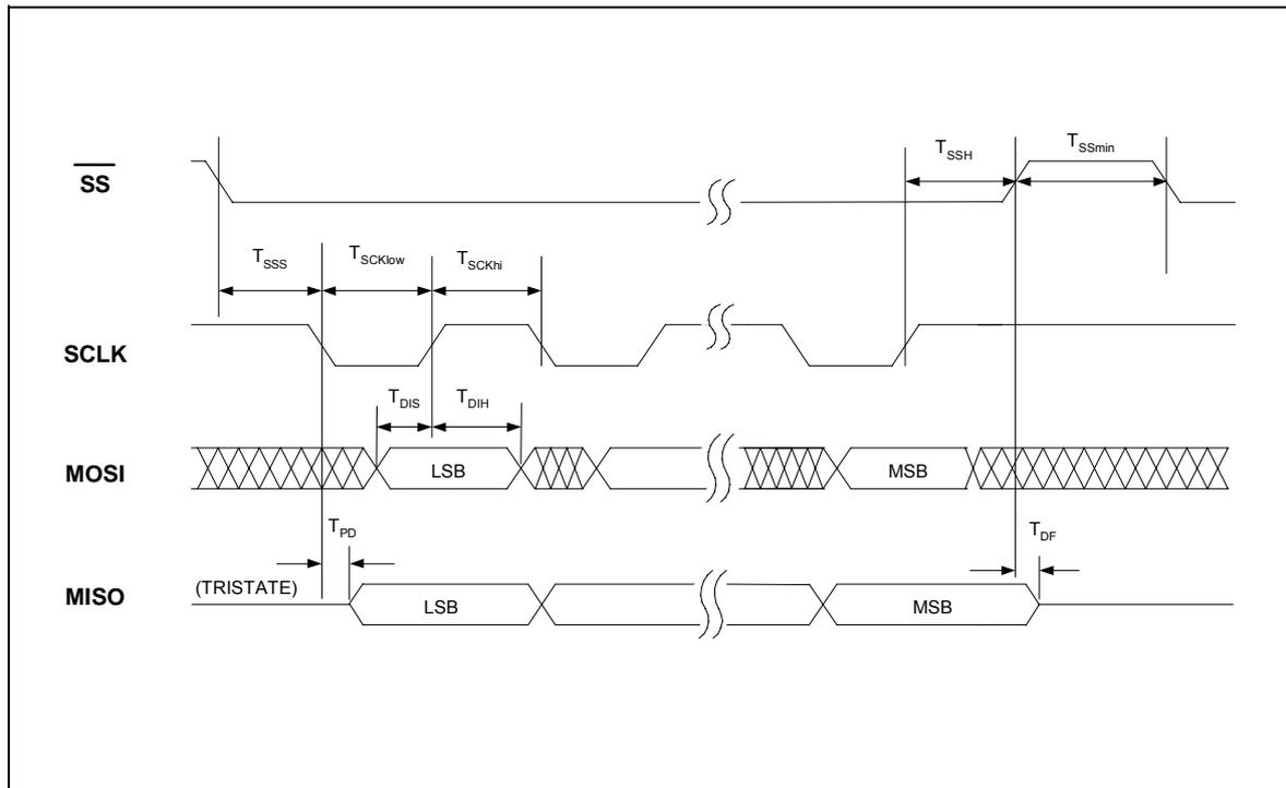
Figure 12.8: SPI Operation
