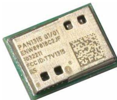
The above pictures show the laser marking on the top case, this is only an example from PAN1315.
