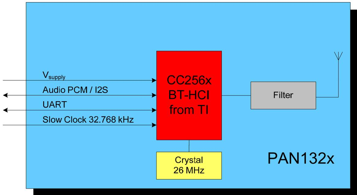
Note: The Slow Clock 32.768 kHz is mandatory, otherwise the module does not start up, refer to Chapter 5.4 for additional information.
