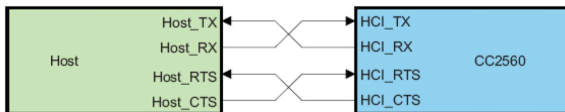
When the UART RX buffer of the CC256X passes the “flow control” threshold, it will set the UART\_RTS signal high to stop transmission from the host.
