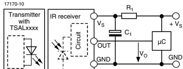
The external components  $R_1$  and  $C_1$  are optional to improve the robustness against electrical overstress (typical values are  $R_1 = 100 \Omega$ ,  $C_1 = 0.1 \mu F$ ).
