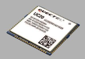
UC20 is the latest Quectel UMTS/ HSPA<sup>+</sup> module offering a maximum data rate of 14.4 Mbps downlink and 5.76 Mbps uplink. UC20 is designed to provide customers with global network coverage on the connectivity of HSPA+/ WCDMA. It can also be fully backward compatible to existing EDGE and GSM/ GPRS networks through multiband combination of quad band WCDMA and quad band GSM.
