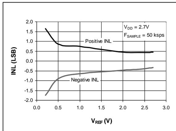
**FIGURE 2-5:** Integral Nonlinearity (INL) vs.  $V_{REF}$  ( $V_{DD} = 2.7V$ ).
