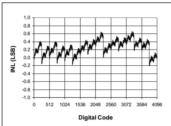
**FIGURE 2-3:** Integral Nonlinearity (INL) vs. Code (Representative Part).
