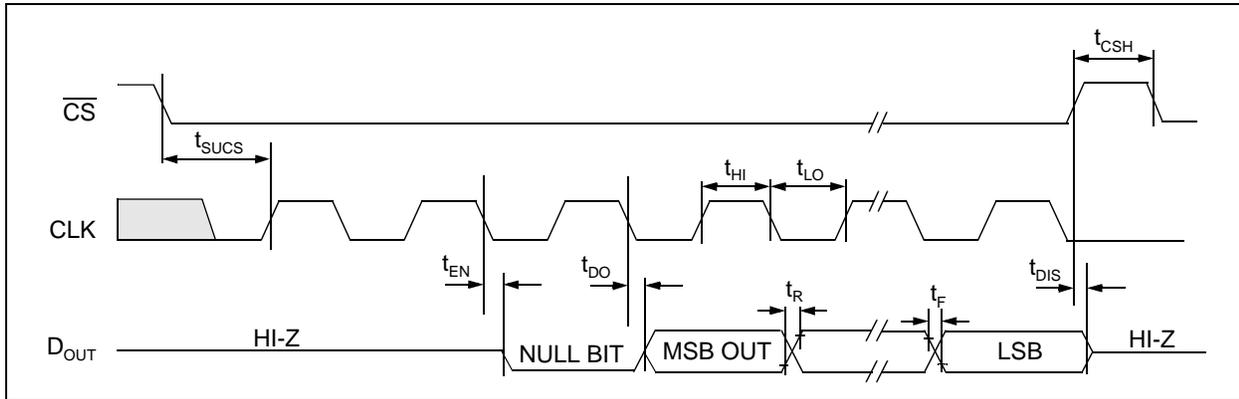
FIGURE 1-1: Serial Timing.
