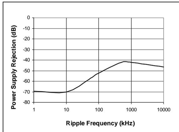
**FIGURE 2-29:** Power Supply Rejection (PSR) vs. Ripple Frequency.
