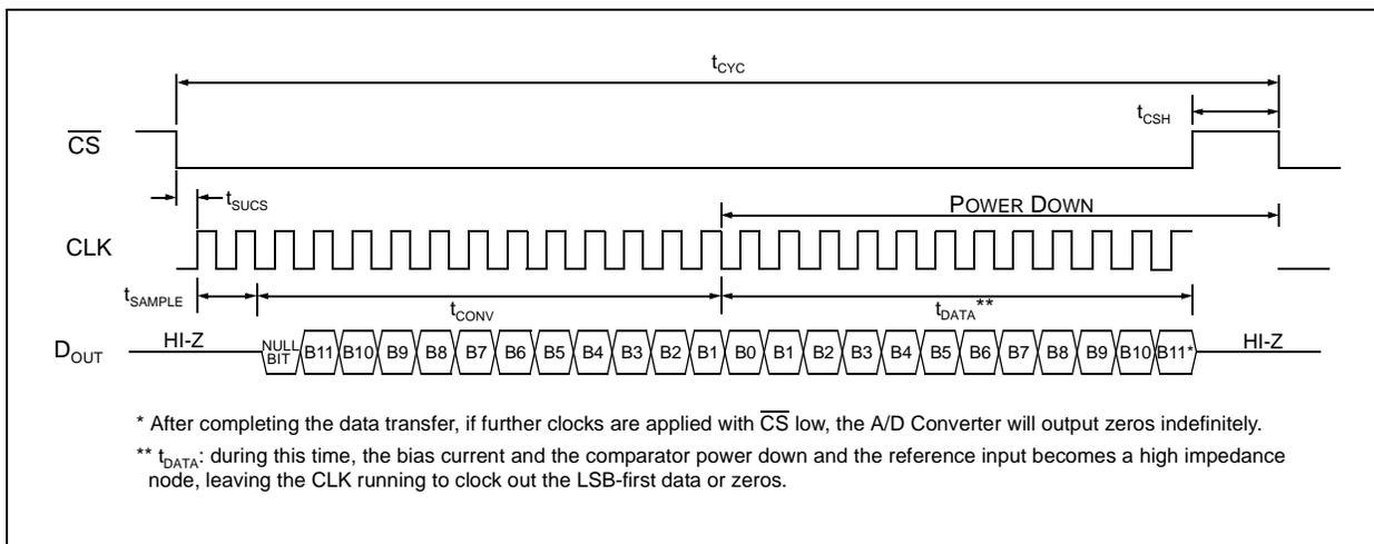
FIGURE 5-2: Communication with MCP3201 using LSB first Format.
