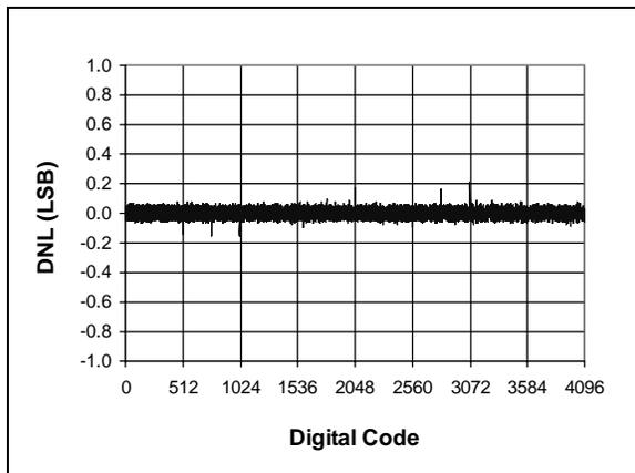
**FIGURE 2-13:** Differential Nonlinearity (DNL) vs. Code (Representative Part).
