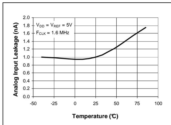
**FIGURE 2-39:** Analog Input Leakage Current vs. Temperature.
