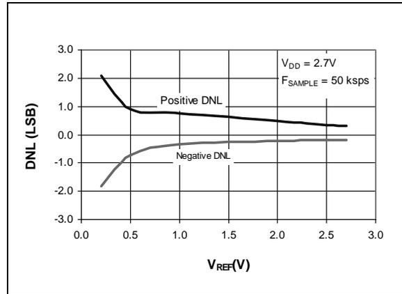
**FIGURE 2-12:** Differential Nonlinearity (DNL) vs.  $V_{REF}$  ( $V_{DD} = 2.7V$ ).
