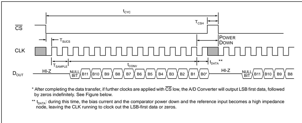
FIGURE 5-1: Communication with MCP3201 using MSB first Format.
