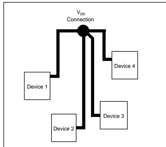
**FIGURE 6-4:** V<sub>DD</sub> traces arranged in a 'Star' configuration in order to reduce errors caused by current return paths.
