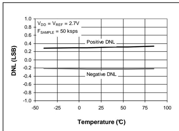
**FIGURE 2-17:** Differential Nonlinearity (DNL) vs. Temperature ( $V_{DD} = 2.7V$ ).
