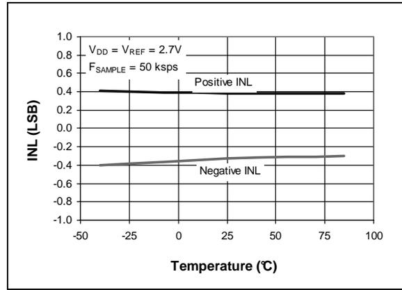
**FIGURE 2-10:** Integral Nonlinearity (INL) vs. Temperature ( $V_{DD} = 2.7V$ ).
