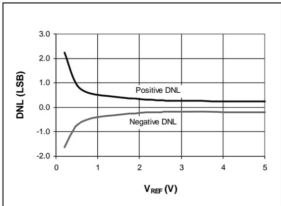
**FIGURE 2-9:** Differential Nonlinearity (DNL) vs.  $V_{REF}$ .
