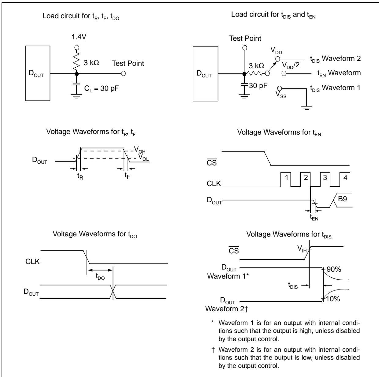
FIGURE 1-2: Test Circuits.
