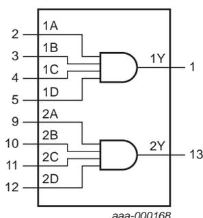
**Fig 1. Functional diagram**
