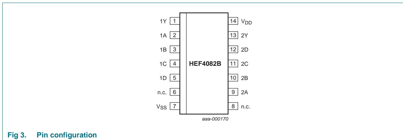
Fig 3. Pin configuration
